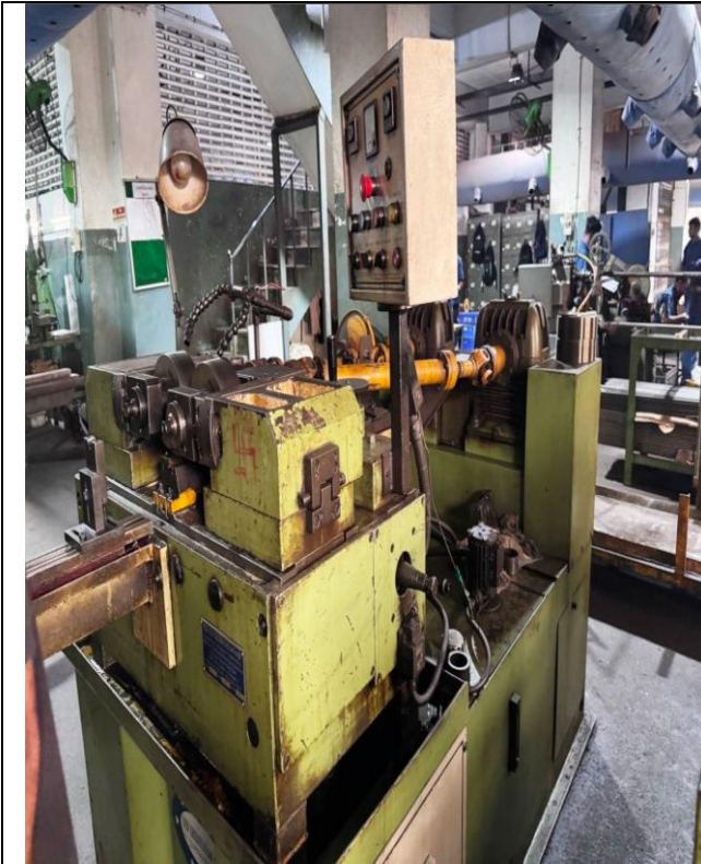
View of Hydraulic Thread Rolling Machine Model TR20 VFD, Sr. No. 54 Installed at Unit-3
