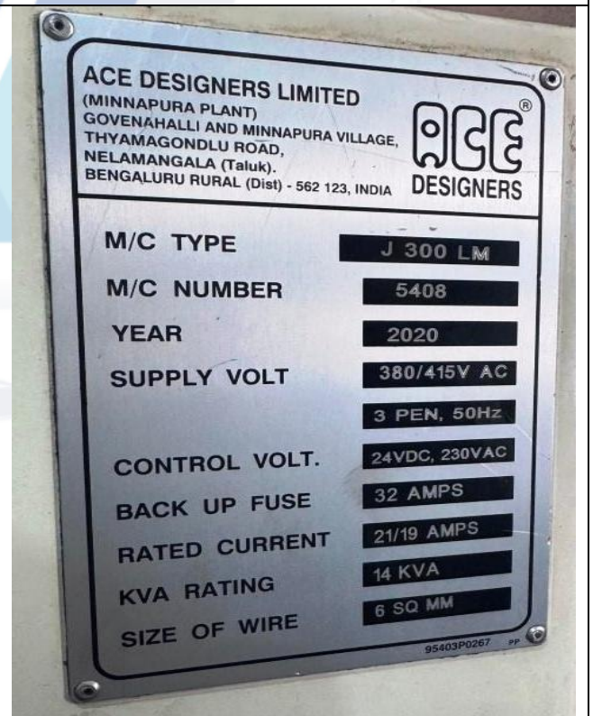
View of Ace CNC Lathe Model: J 300LM, Sr. No. 5408 Installed at Unit-3
