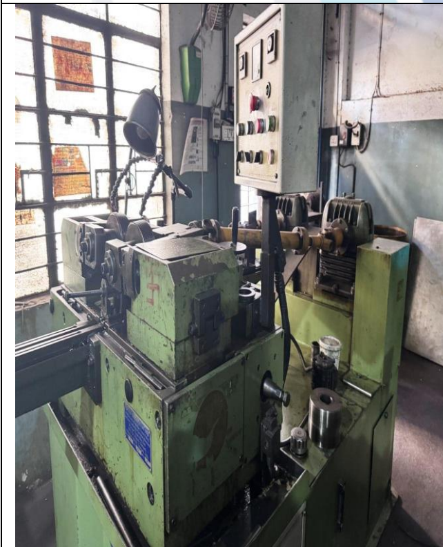
View of Hydraulic Thread Rolling Machine Model TR20 VFD, Sr. No. 55 Installed at Unit-3
