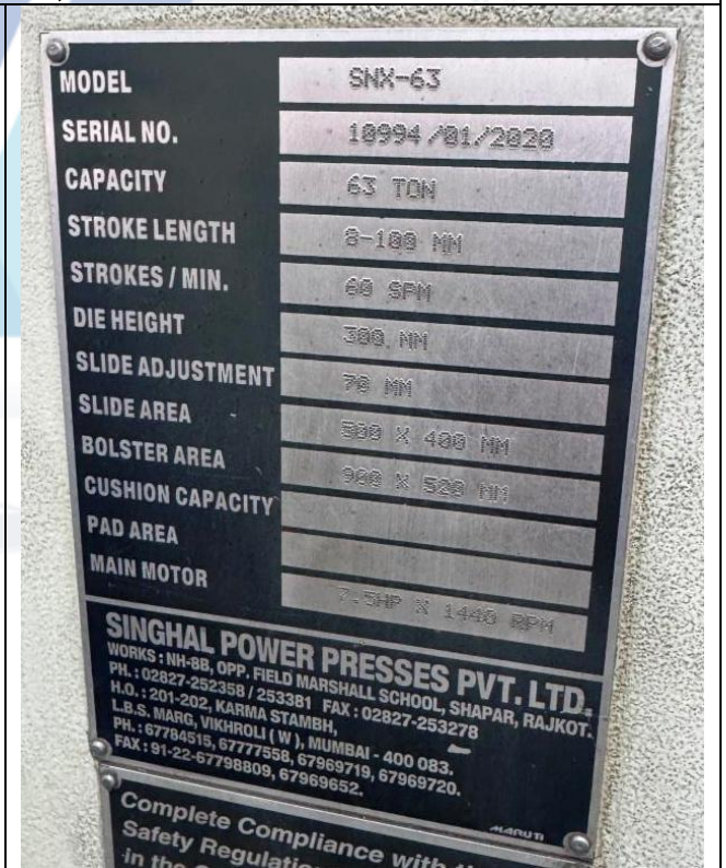
View of Sewcross Shaft Geared Power Press Complete with Standard Accessories, Model SNX 63T (SG), Sr. No. 10994/01/2020 Installed at Unit-4
