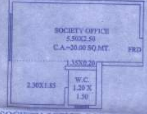
BUA DIAGRAM (TYPICAL FLOOR) 2ND TO 7TH, 9TH TO 14TH, 16TH TO 21ST, 23RD TO 25TH FLOOR SCALE 1:100
