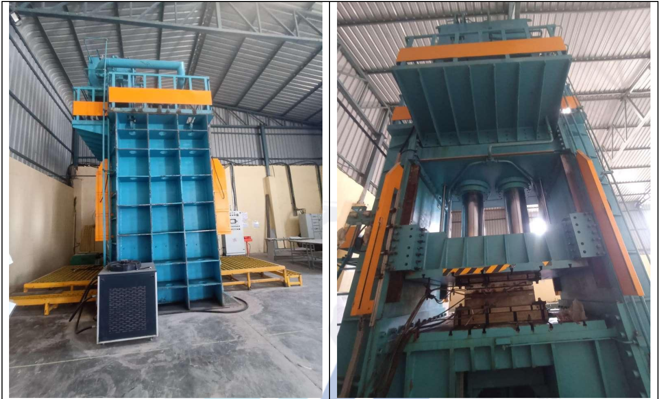
View of Santec make Hydraulic Moulding Press Model-SMC 600 Ton, Sr. No. SE-21-22-U5-09
