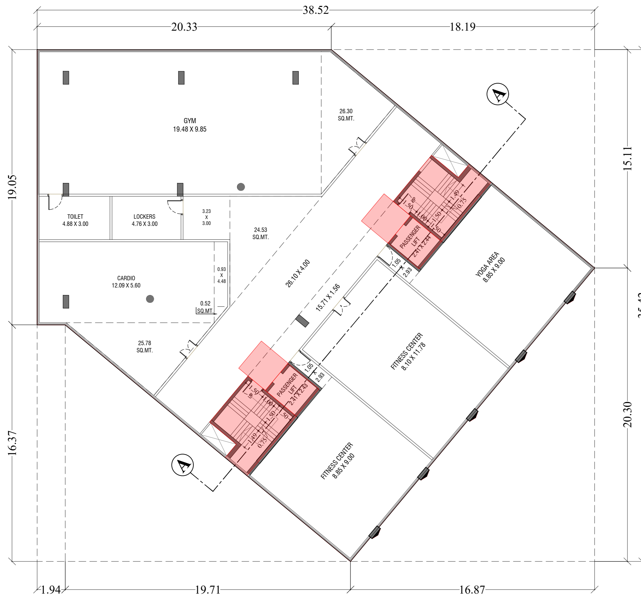
FIRST FLOOR PLAN (FITNESS CENTER) SCALE - 1:100
