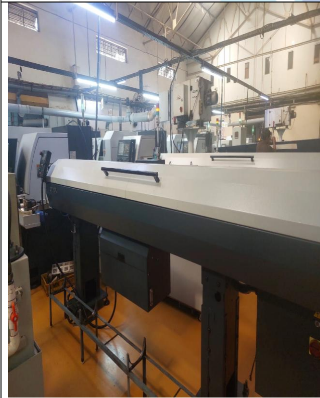
Automatic Bar Feeder, Model- GT 342, Length-3.2 Mtrs.
