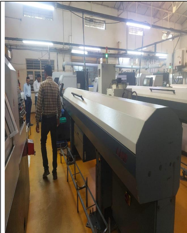
Automatic Bar Feeder, Model- GT 342, Length-3.2 Mtrs.
