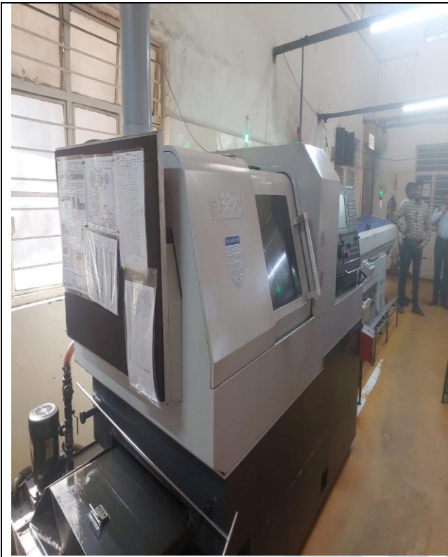
Nexturn Swiss Type Sliding Head Machine with Standard Accessories, Model- SA32PII
