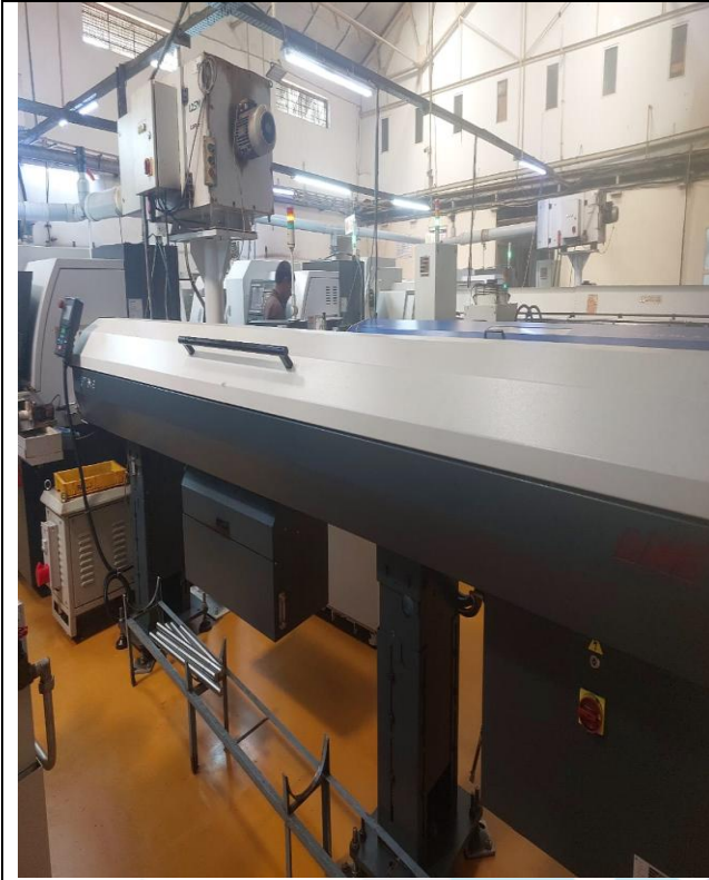
Automatic Bar Feeder, Model- GT 342, Length-3.2 Mtrs.
