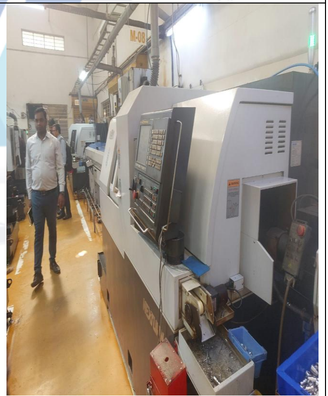
Nexturn Swiss Type Sliding Head Machine with Standard Accessories, Model- SA32PII
