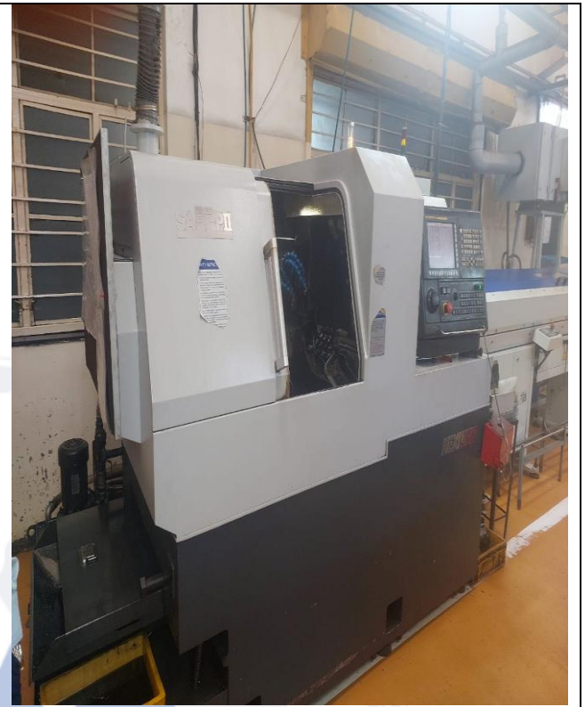
Nexturn Swiss Type Sliding Head Machine with Standard Accessories, Model- SA32PII
