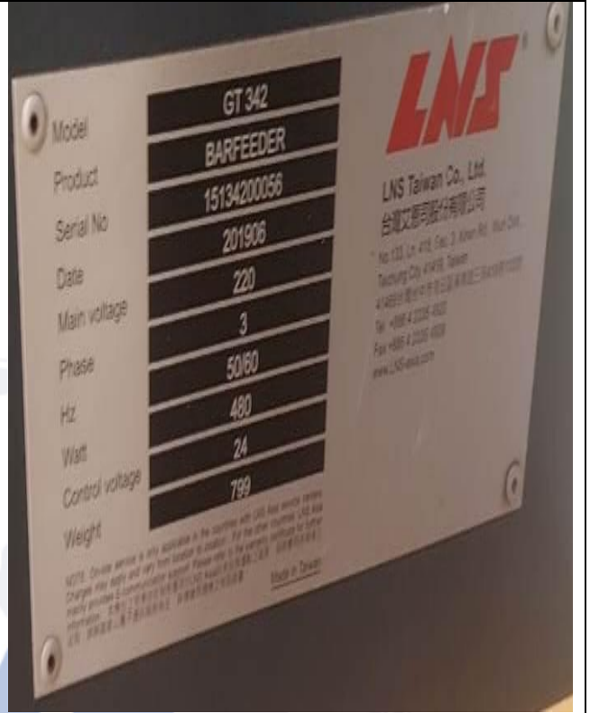
Automatic Bar Feeder, Model- GT 342, Length-3.2 Mtrs.
