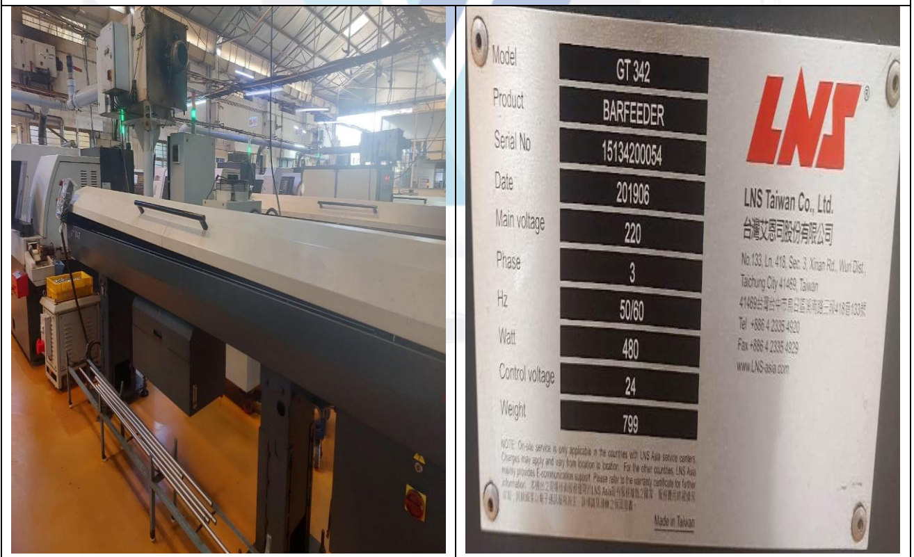
Automatic Bar Feeder, Model- GT 342, Length-3.2 Mtrs.
