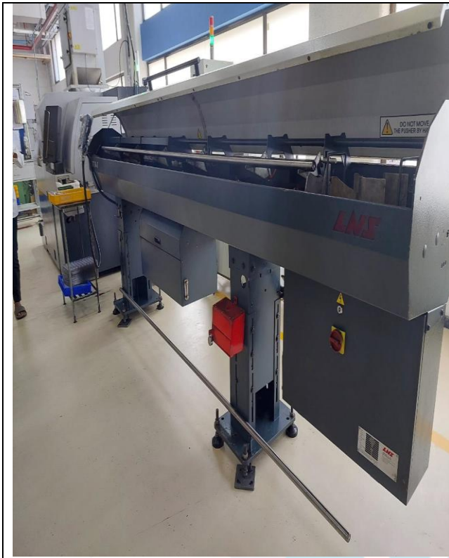
Automatic Bar Feeder, Model- GT 342, Length-3.2 Mtrs.
