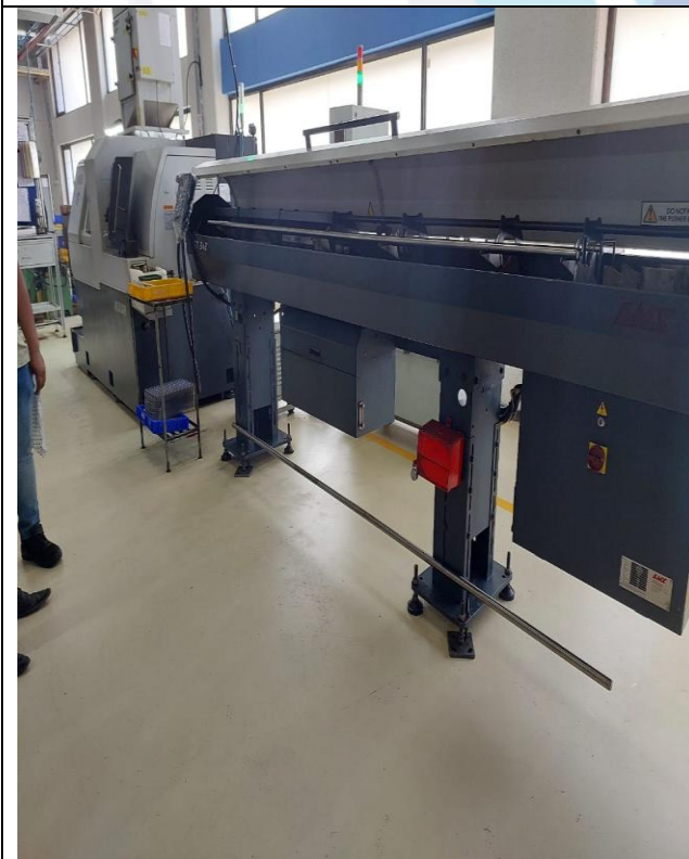
Automatic Bar Feeder, Model- GT 342, Length-3.2 Mtrs.
