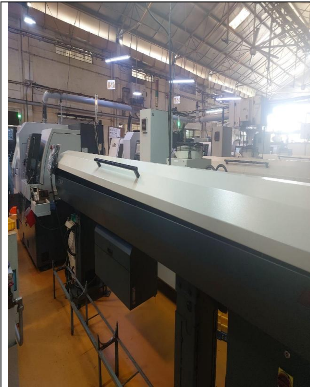
Automatic Bar Feeder, Model- GT 342, Length-3.2 Mtrs.
