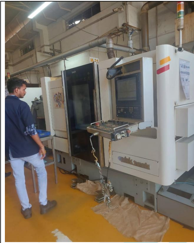
CNC Multi-tasking turning Center with milling function, Sr. No. 4537
