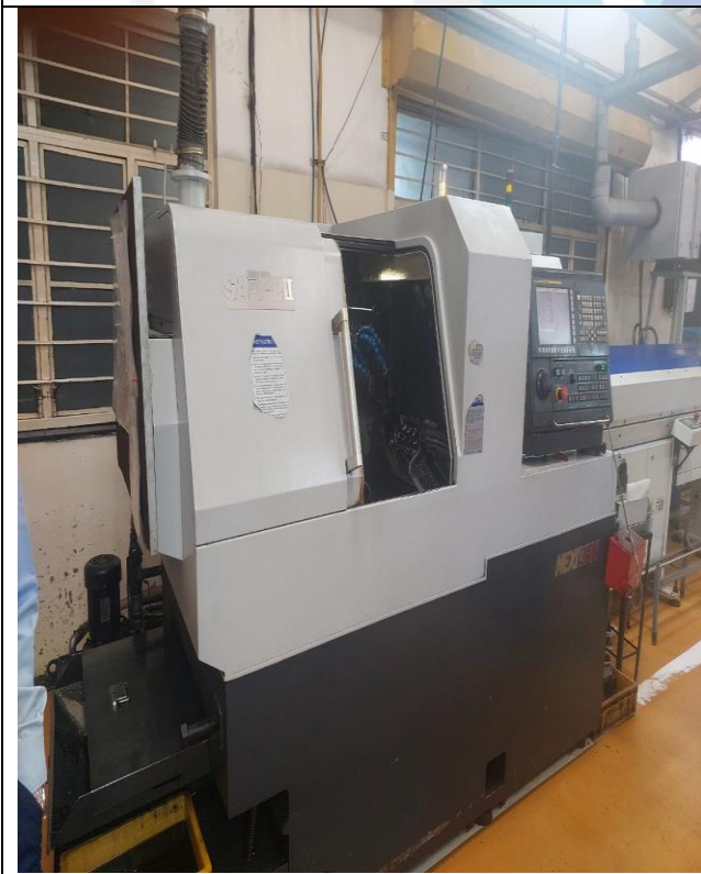
Nexturn Swiss Type Sliding Head Machine with Standard Accessories, Model- SA32PII
