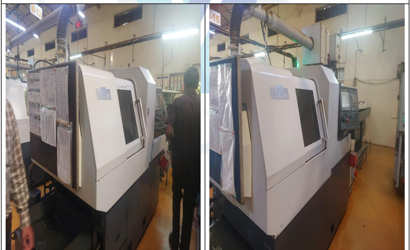
Nexturn Swiss Type Sliding Head Machine with Standard Accessories, Model- SA32PII
