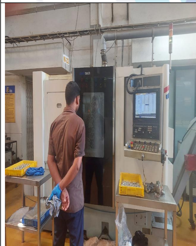
CNC Multi-tasking turning Center with milling function, Sr. No. 4547
