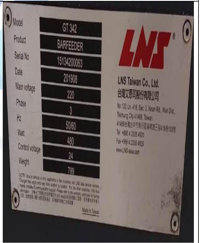
Automatic Bar Feeder, Model- GT 342, Length-3.2 Mtrs.
