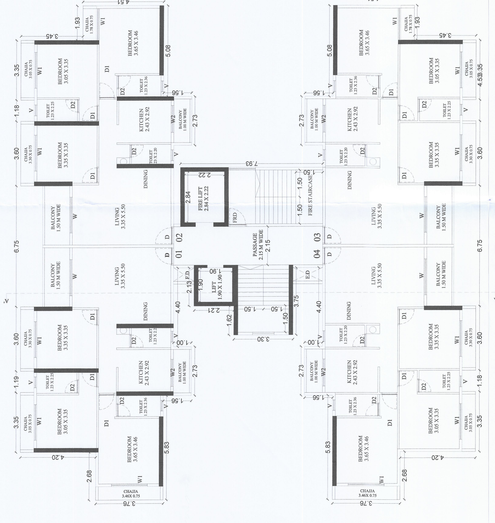
4TH TO 7TH, 9TH TO 12TH & 14TH TO 17TH FLOOR PLAN (SCALE 1:100)
