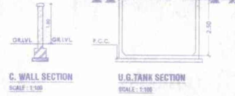
C. WALL SECTION SCALE = 1:100
