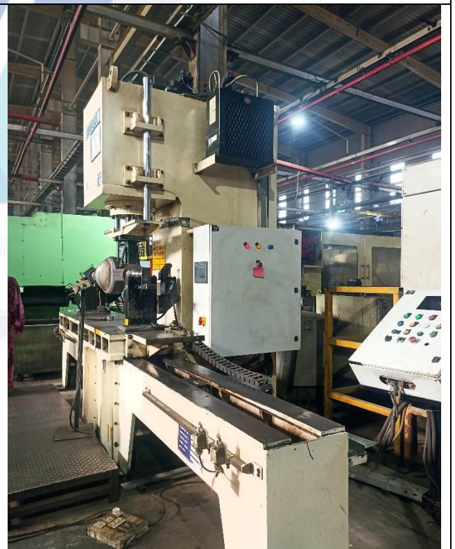
100 T C Frame Hydraulic Press (SEAPL) with Accessories
