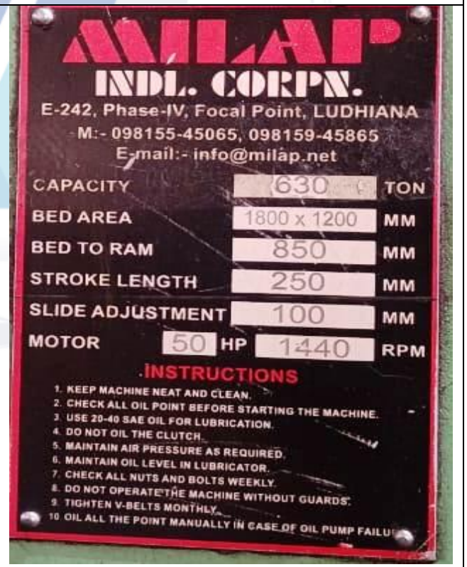
Milap make Power Press 630 Tons Capacity Steel body H Frame and Crank UT Test
