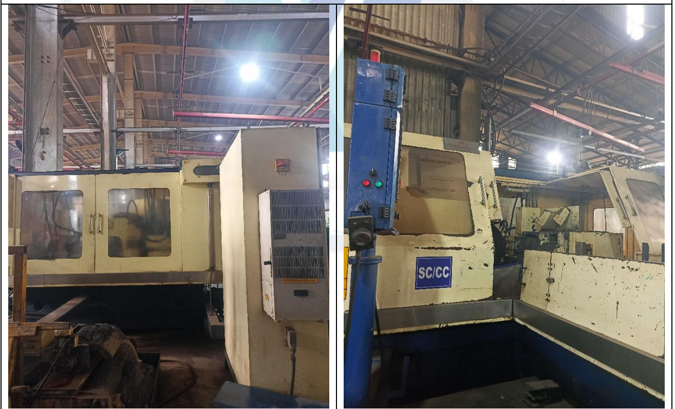
VMPL make 9 Axis Angular head CNC Center less grinding Machine
