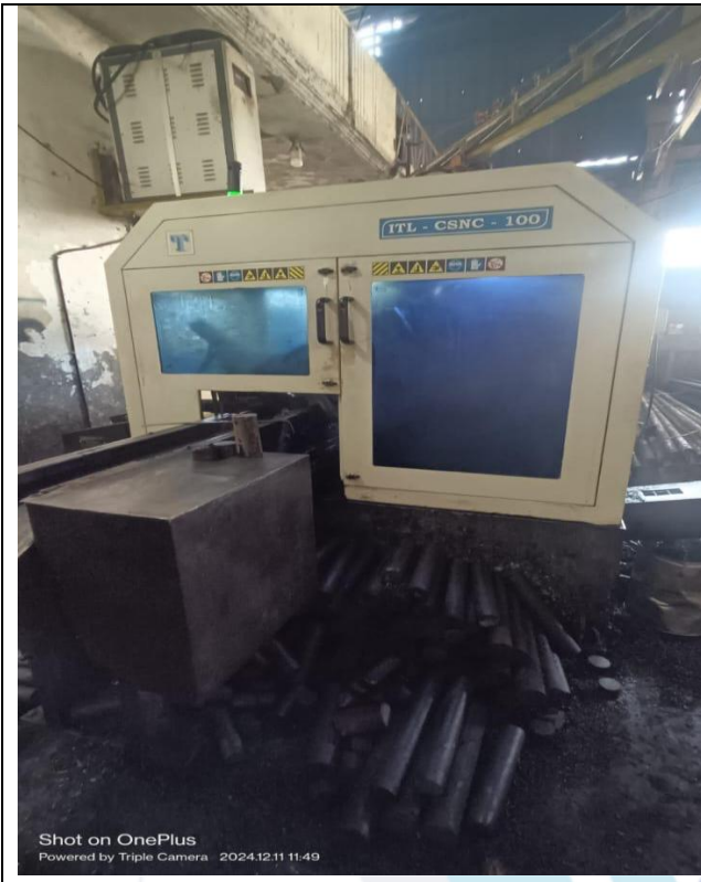
High Speed Circular Saw, Model-ITL CSNC-100
