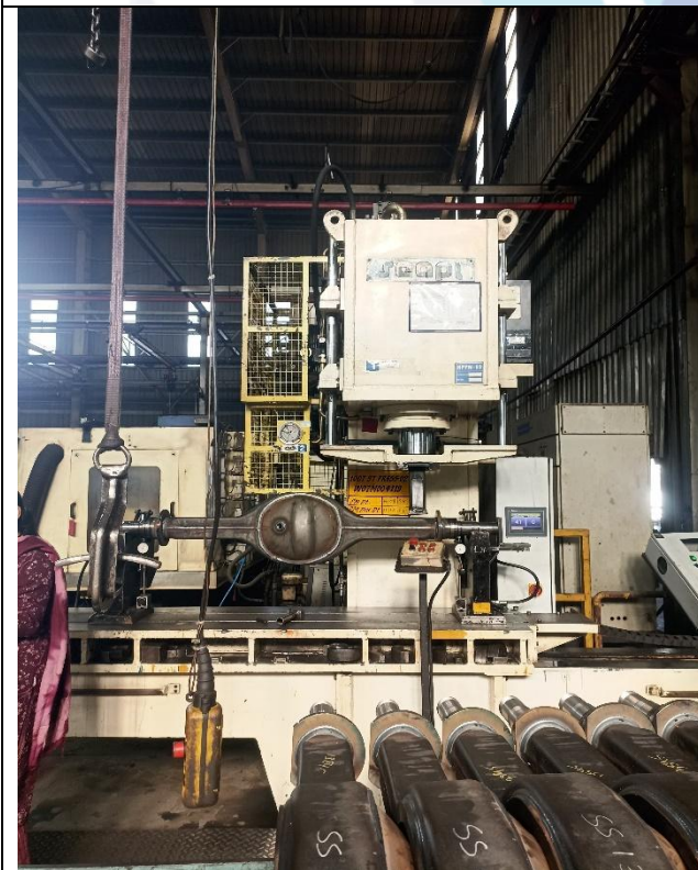
100 T C Frame Hydraulic Press (SEAPL) with Accessories
