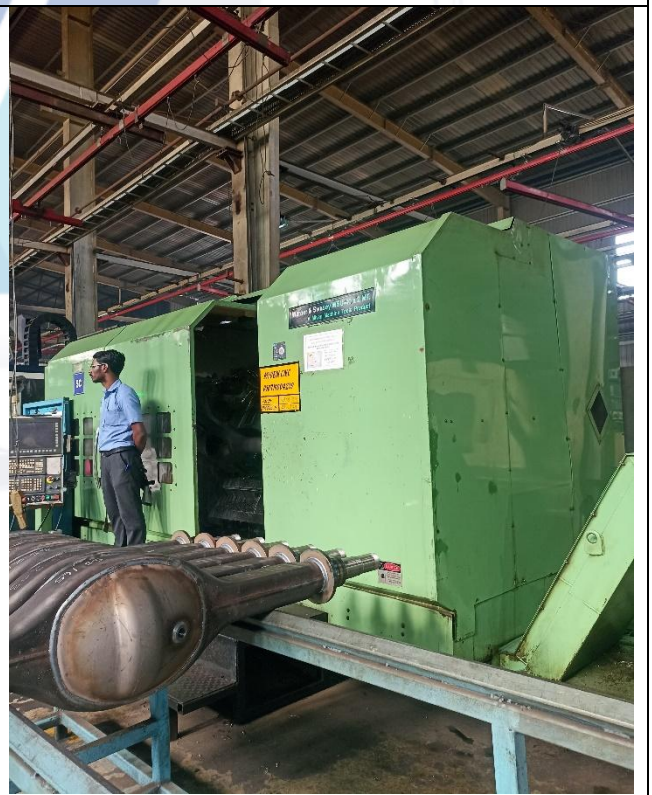
WSU-40 X 2200 mm, Slant Bed CNC Turning Machine Centre with Standard Accessories
