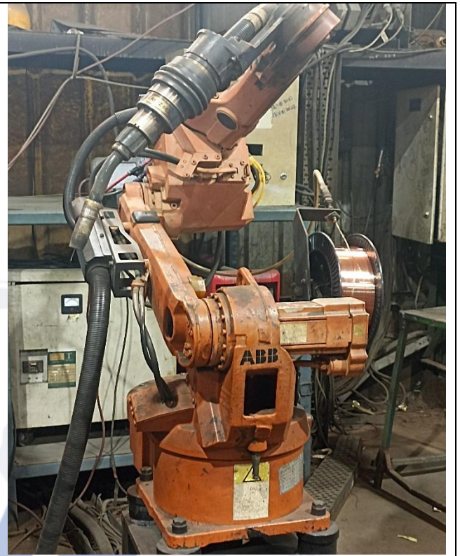
Industrial Robot System, IRB 1520 with MTD 500
