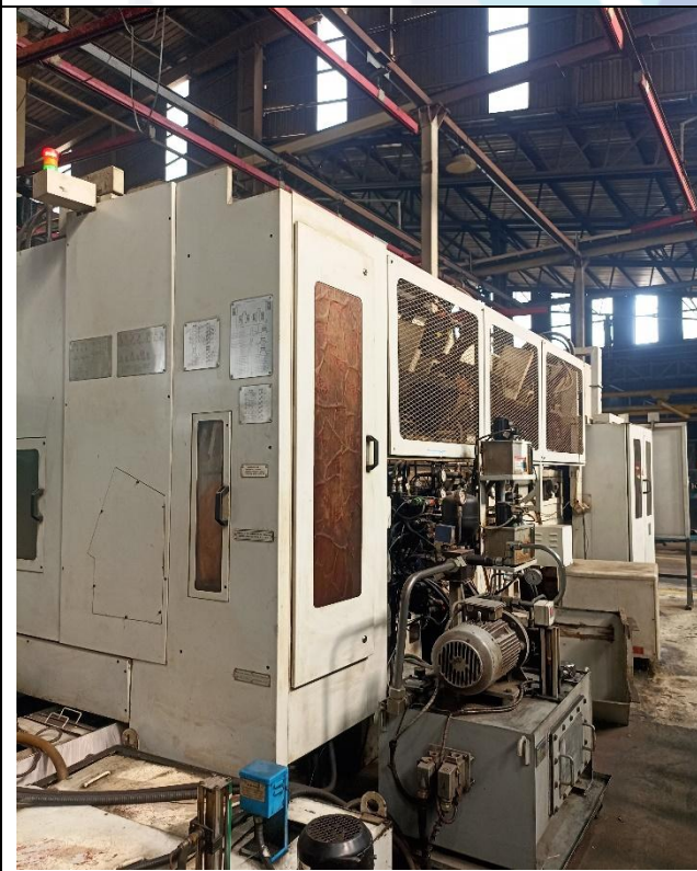
BFW (proteck) heavy duty twin carriage 5 axis slant Bed CNC turn-mill centre,
