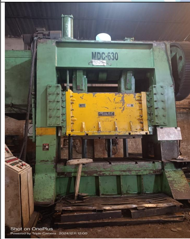
Milap make Power Press 630 Tons Capacity Steel body H Frame and Crank UT Test
