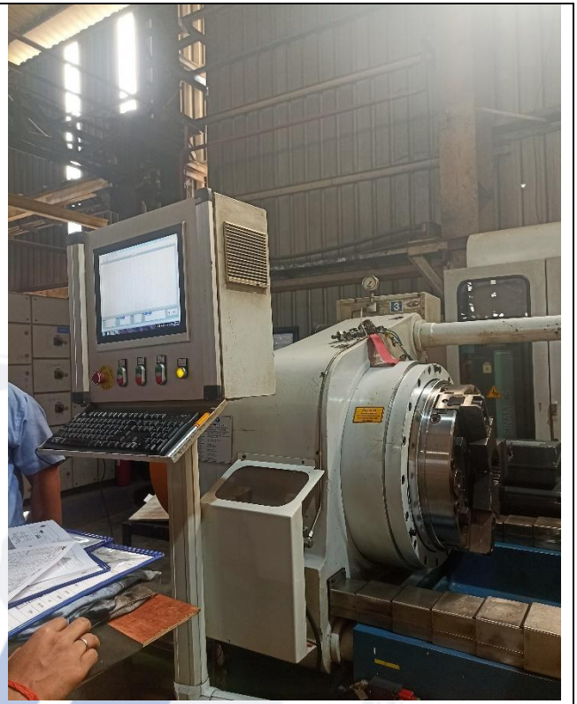
WF170/100 Ton Horizontal Single Head Friction Welding Machine with orientation
