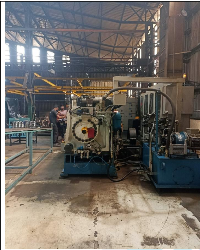
WF170/100 Ton Horizontal Single Head Friction Welding Machine with orientation
