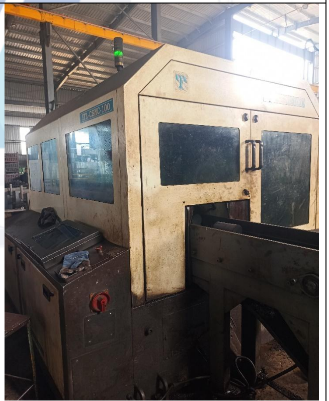
High Speed Circular Saw, Model-ITL CSNC-100
