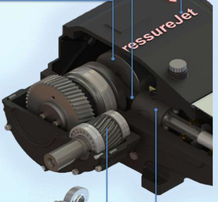
Integrated gear unit (alloy steel)
