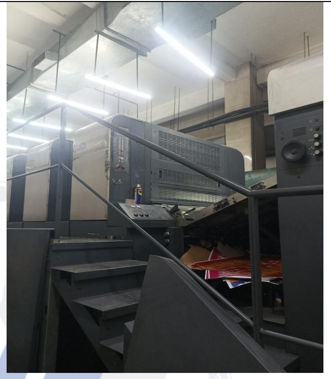
High Capacity Eight Colour Sheetfed Offset Press, Model- Roland 708 LV Evolution Size 3B,
