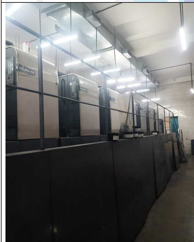
High Capacity Eight Colour Sheetfed Offset Press, Model- Roland 708 LV Evolution Size 3B,
