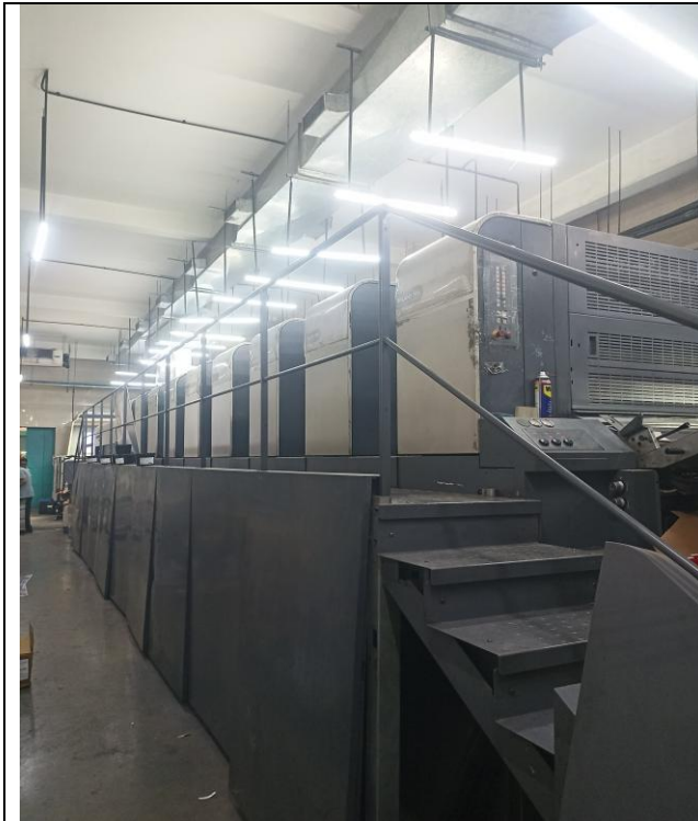
High Capacity Eight Colour Sheetfed Offset Press, Model- Roland 708 LV Evolution Size 3B,
