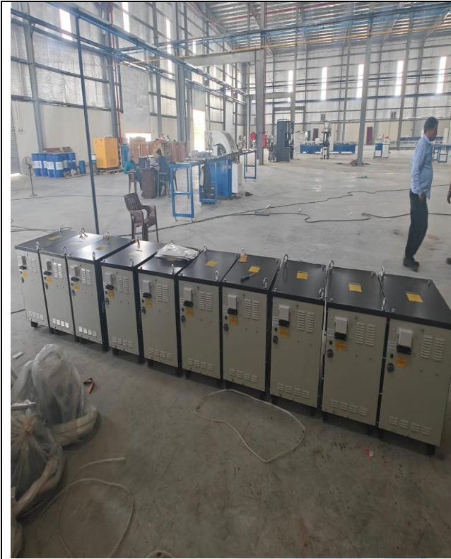
View of KRII400 Amp Panasonic Make thristor Mig Welding MC with Accessories- Kept in Shed
