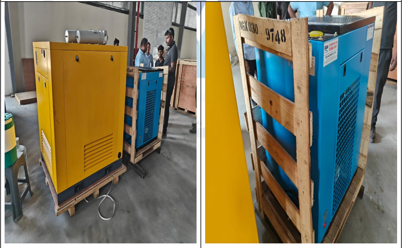
View of First Air Make 50HP Oil lubricated Rotary Screw Air Compressor with Dryer, Filter, Air Receiver Tank- Partially kept in box
