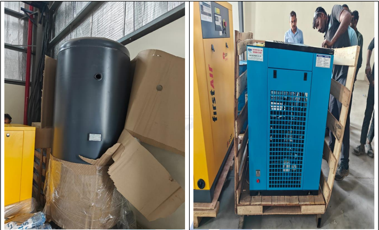
View of First Air Make 50HP Oil lubricated Rotary Screw Air Compressor with Dryer, Filter, Air Receiver Tank- Partially kept in box
