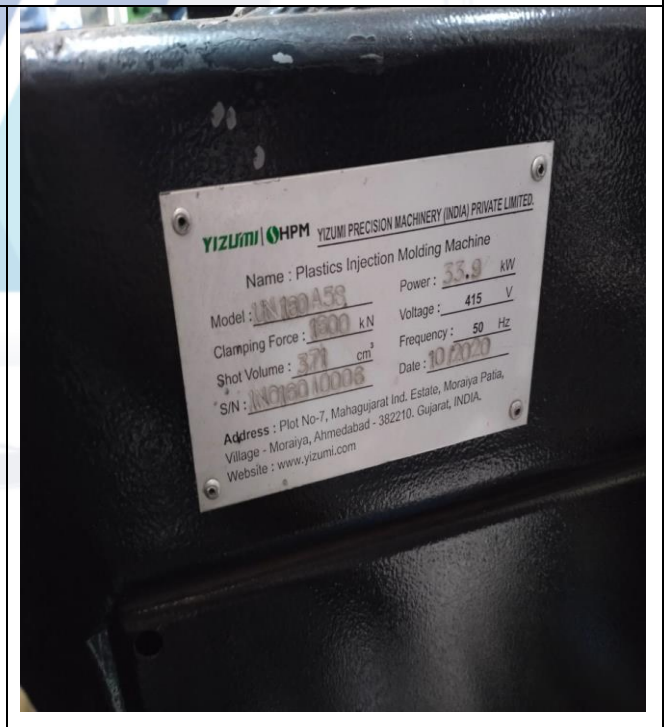
3 Platen Toggle Injection Moulding Machine, Locking Force-160 Ton, Screw Dia. 48 mm (Type-B), Sr. No. IN16010006
