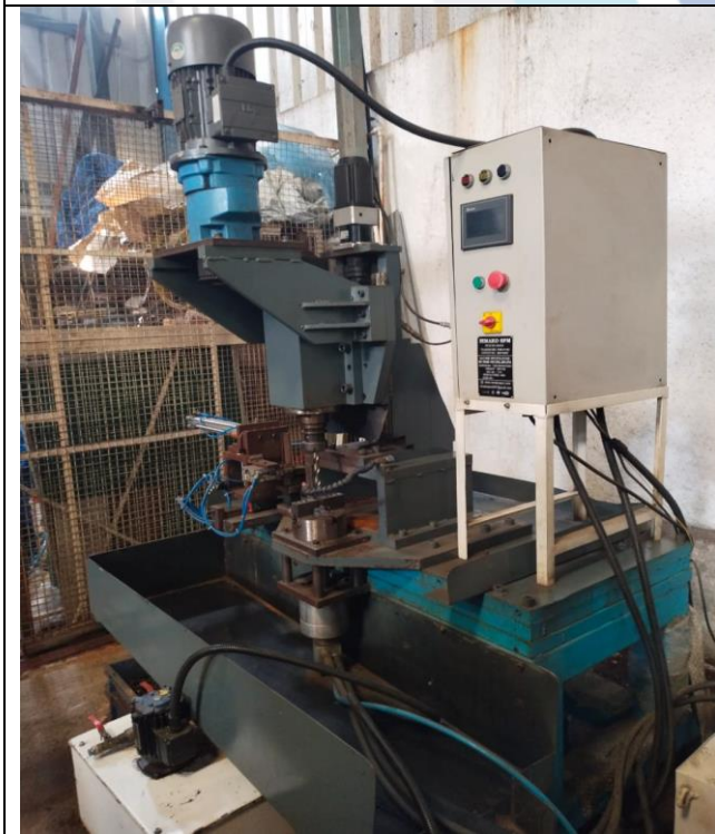
Drilling SPM Single Spindle with pick and place
