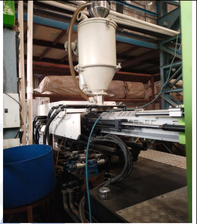
3 Platen Toggle Injection Moulding Machine, Locking Force-260 Ton, Screw Dia. 60 mm (Type-B), Sr. No. IN026010007
