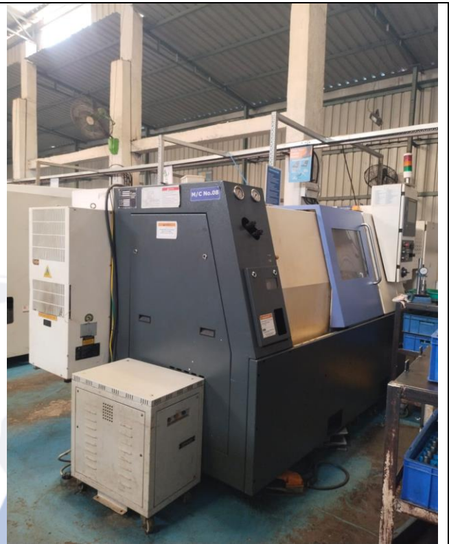
Jyoti make CNC, Model SPM-200-3A with Fanuc Controller & all standard Accessories and Electricals, Sr. No. 60033015-2021
