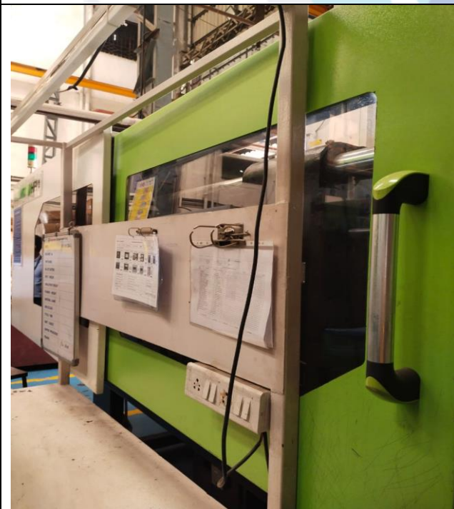
3 Platen Toggle Injection Moulding Machine, Locking Force-260 Ton, Screw Dia. 60 mm (Type-B), Sr. No. IN026010007
