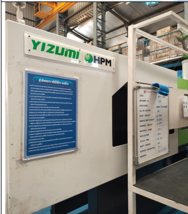
3 Platen Toggle Injection Moulding Machine, Locking Force-160 Ton, Screw Dia. 48 mm (Type-B), Sr. No. IN16010006
