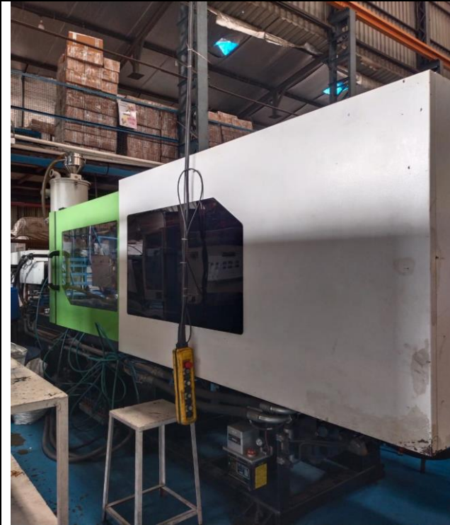
3 Platen Toggle Injection Moulding Machine, Locking Force-260 Ton, Screw Dia. 60 mm (Type-B), Sr. No. IN026010007
