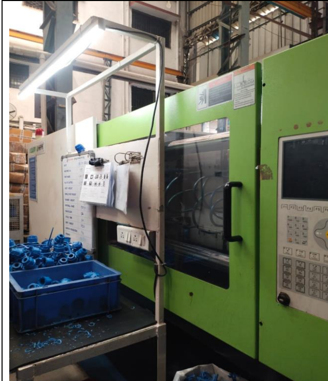
3 Platen Toggle Injection Moulding Machine, Locking Force-200 Ton, Screw Dia. 53 mm (Type-B), Sr. No. IN0200H0022
