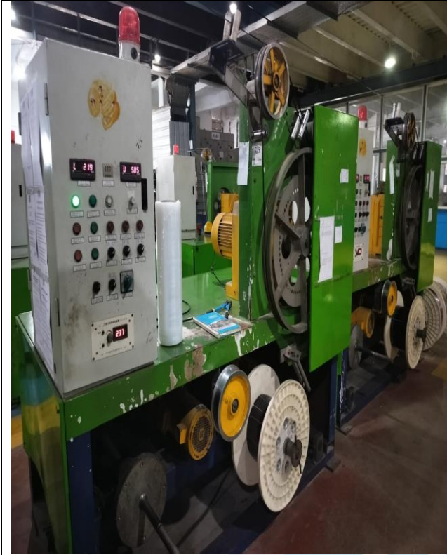
QHLF4/2-3+3/12 Type Flat Wire Enamelling Machine
