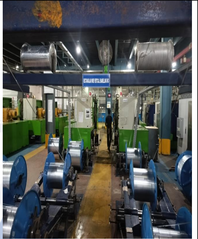
QHLF4/2-3+3/12 Type Flat Wire Enamelling Machine
