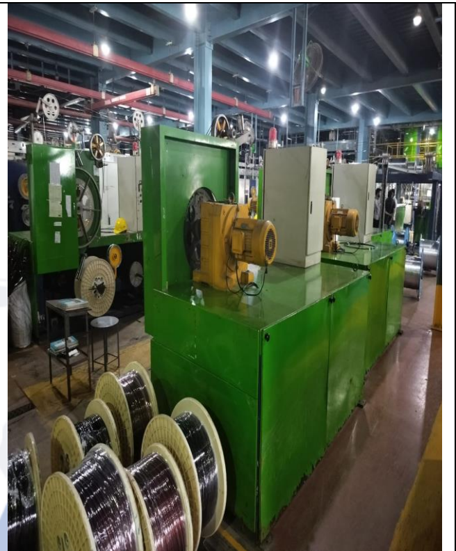
QHLF4/2-3+3/12 Type Flat Wire Enamelling Machine
