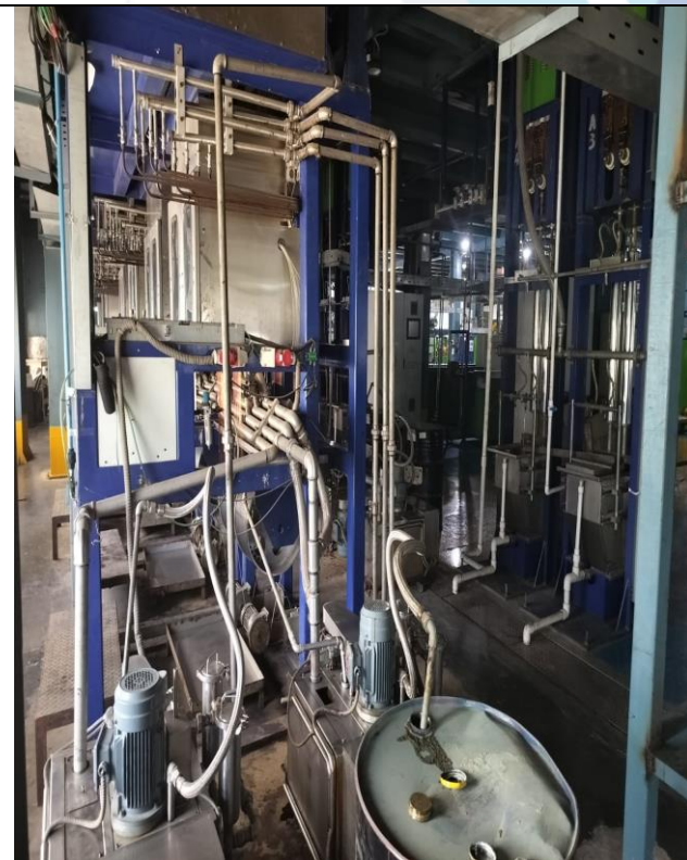
QHLF4/2-3+3/12 Type Flat Wire Enamelling Machine
