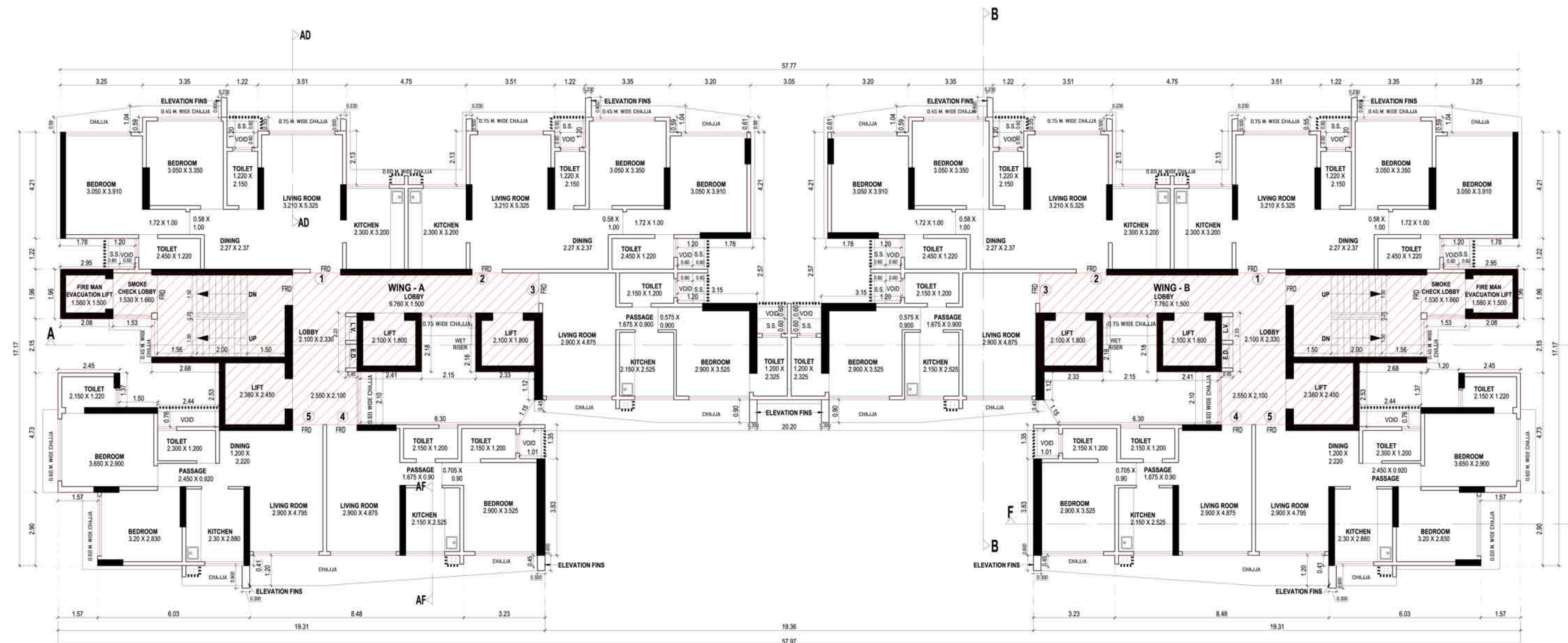
WING - A & B TYPICAL FLOOR PLAN (4TH & 5TH, 7TH TO 11TH FLOORS) SCALE-1:100
