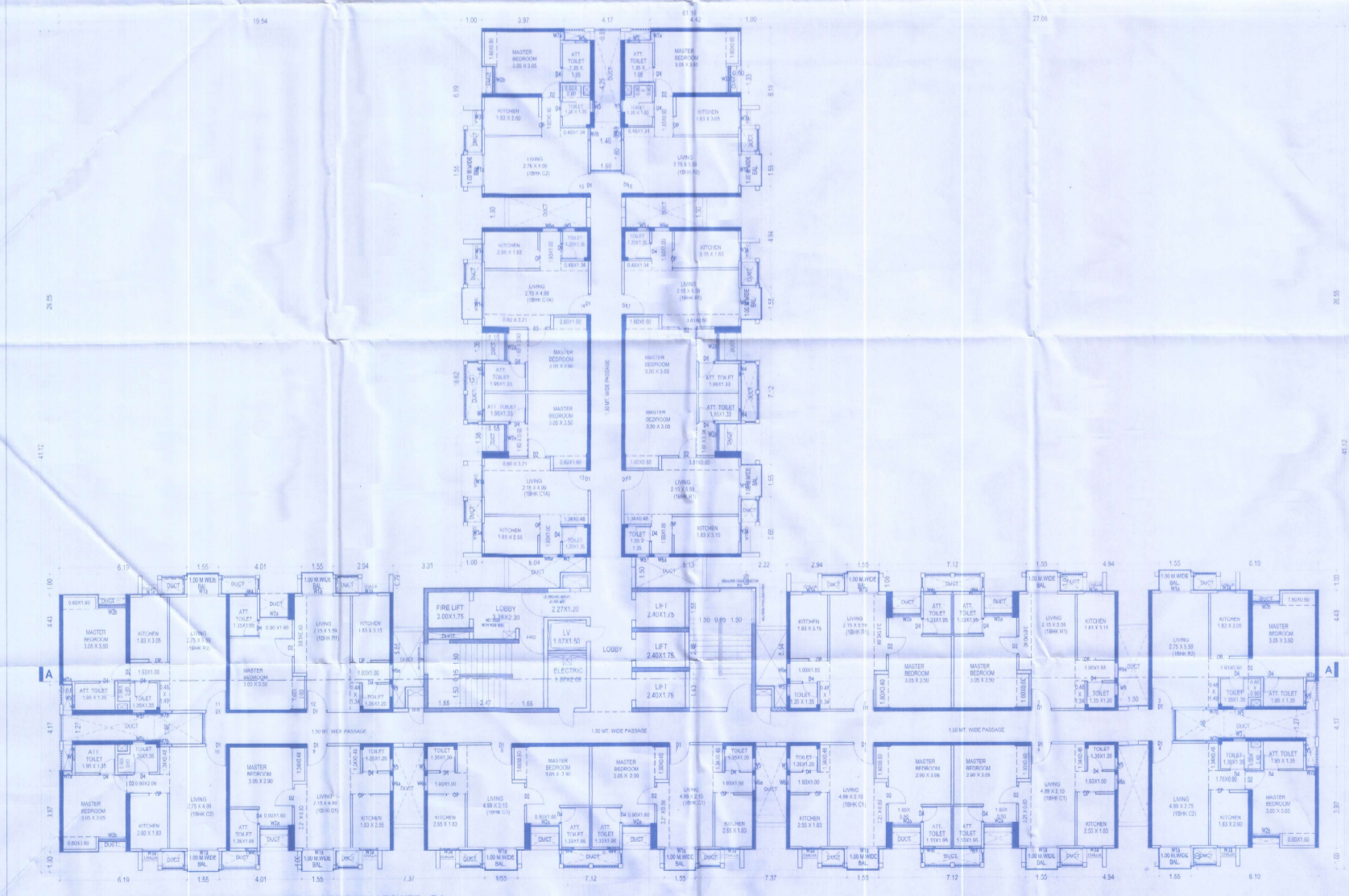
2ND TO 8TH, 10TH TO 14TH TYPICAL FLOOR PLAN ( TOWER - D ) SCALE: 1:100
