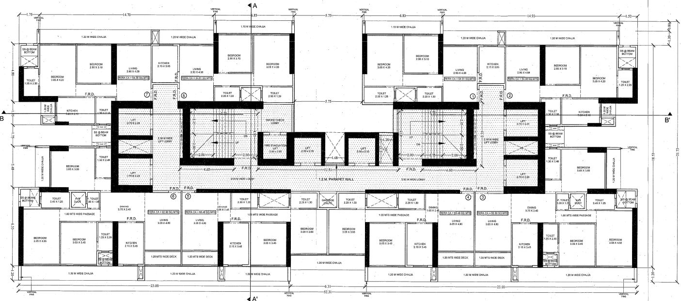
TYPICAL FLOOR PLAN (13TH TO 14TH, 16TH TO 21ST, 23RD TO 28TH, 30TH TO 35TH, 37TH TO 42ND, 44TH) SCALE: 1:100
