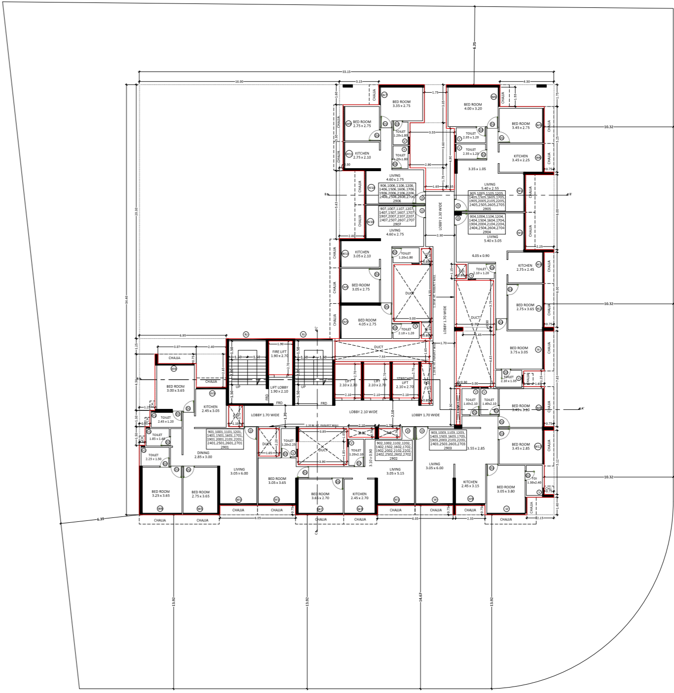
9TH, 10TH, 11TH, 12TH, 14TH, 15TH, 16TH, 17TH, 19TH, 20TH, 21ST, 22ND, 24TH, 25TH, 26TH, 27TH, 29TH FLOOR PLAN SCALE 1:100
