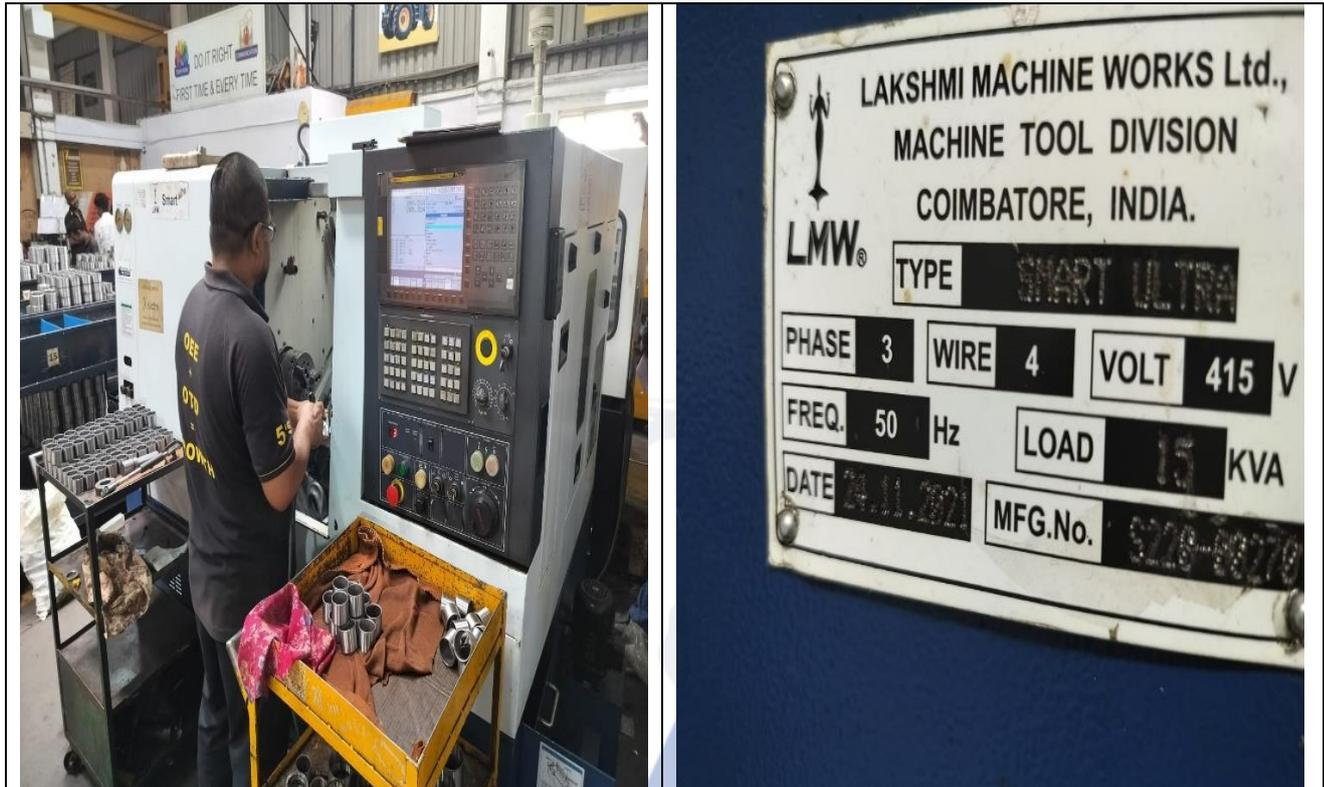
Smart Ultra CNC Lathe- Fanuc, Sr. No. S220-00270-Installed at Unit-II
