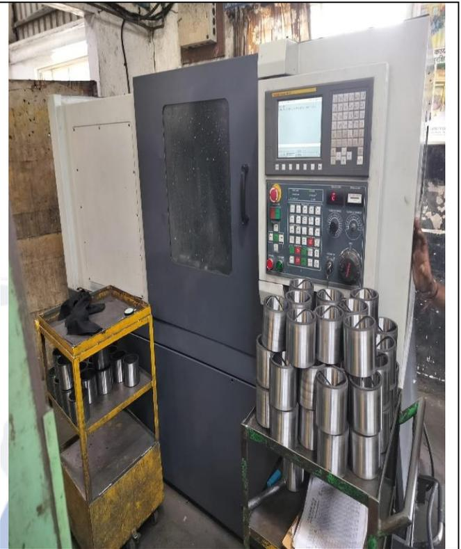
**CNC Turning Centre Lathe, Model-Turbo Turn TT-5 with attached Fixture with Electrical Cabinet and Pendent-Installed at Unit-II**
