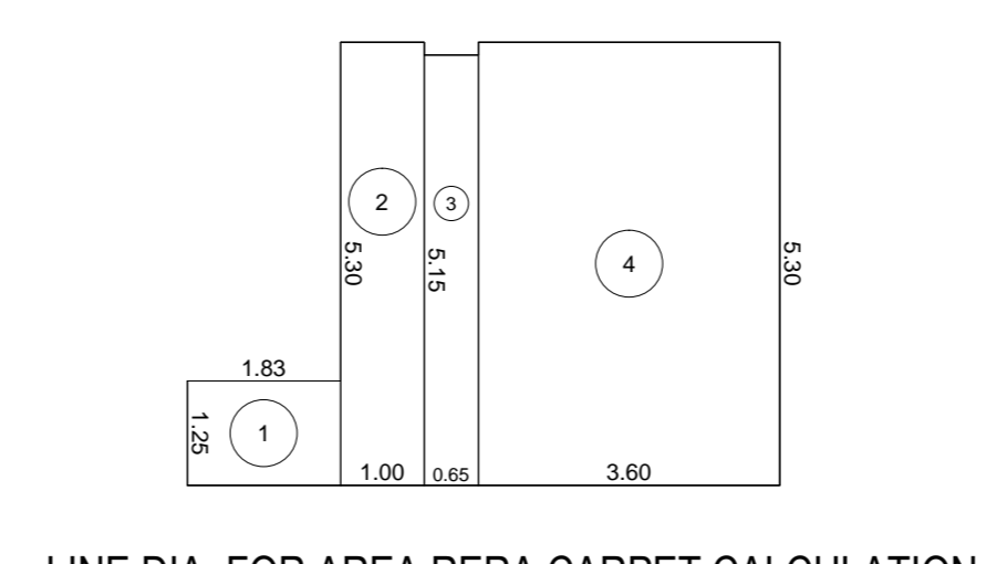
LINE DIA. FOR AREA RERA CARPET CALCULATION OF TYPICAL(4TH TO 6TH) FLOOR (B-WING) SCALE:1:100
