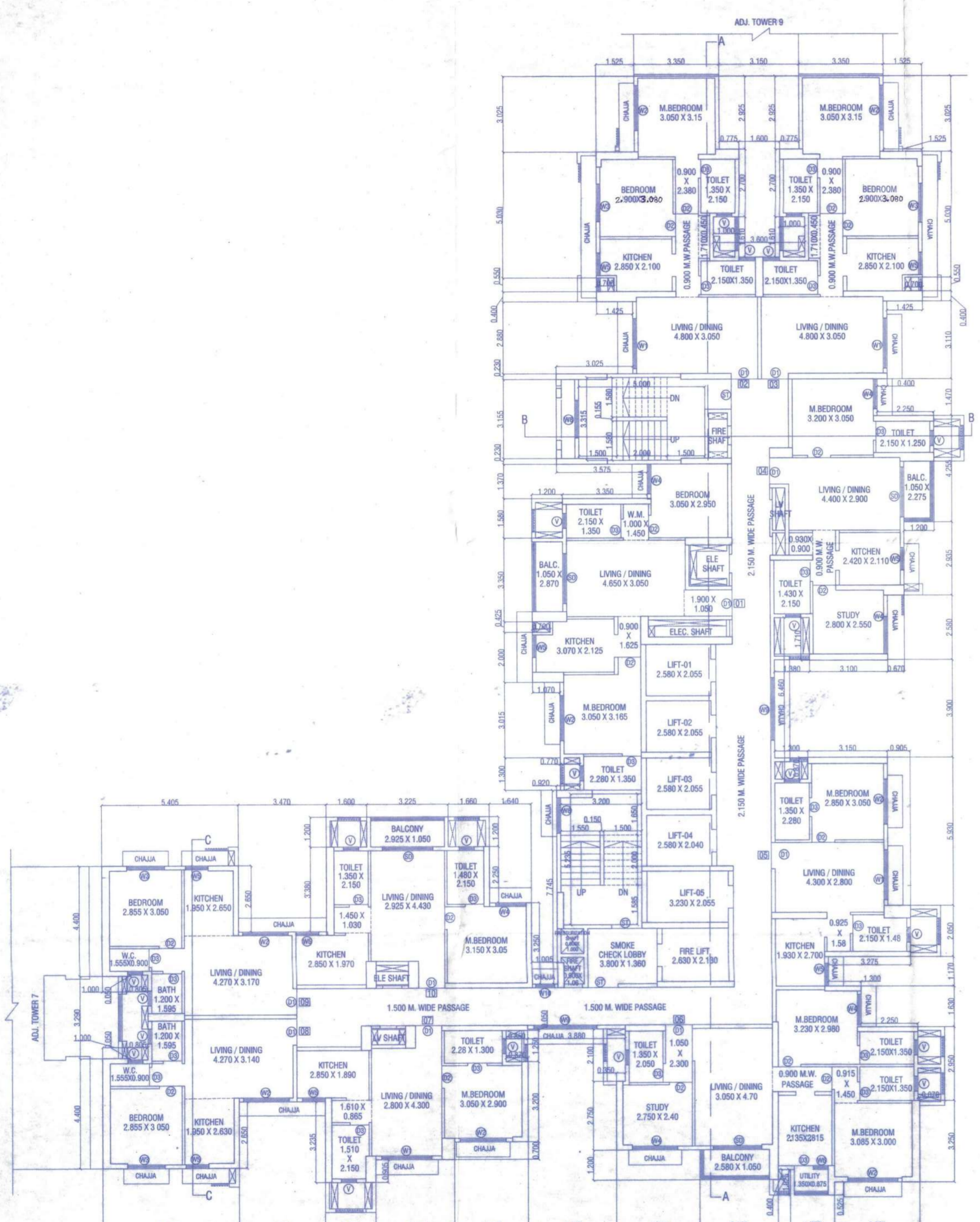
TYPICAL 2ND TO 7TH, 9TH TO 12TH, 14TH TO 17TH, 19TH TO 22ND, 24TH TO 27TH, 29TH TO 32ND FLOOR PLAN SCALE: 1:100
