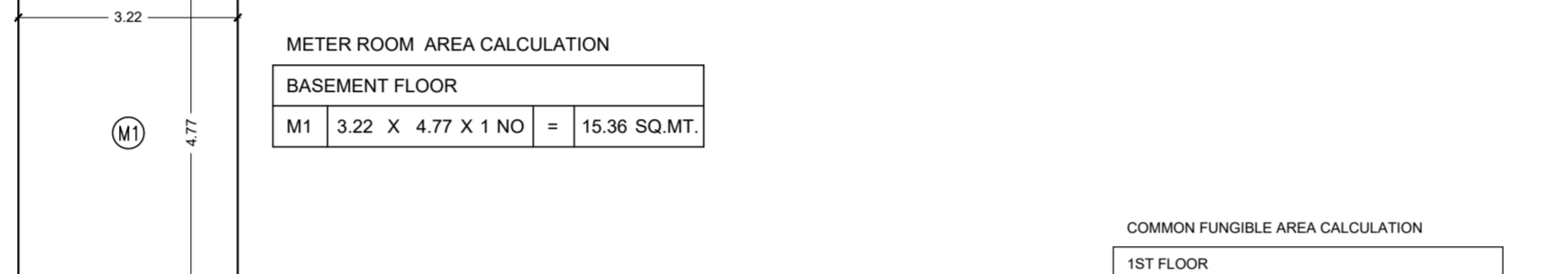
METER ROOM AREA LINE DIAGRAM SCALE 1:100
