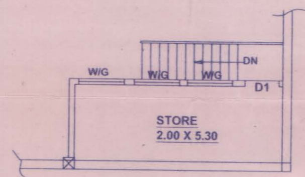
MEZZANINE FLOOR PLAN (ABOVE TOILET AREA)
