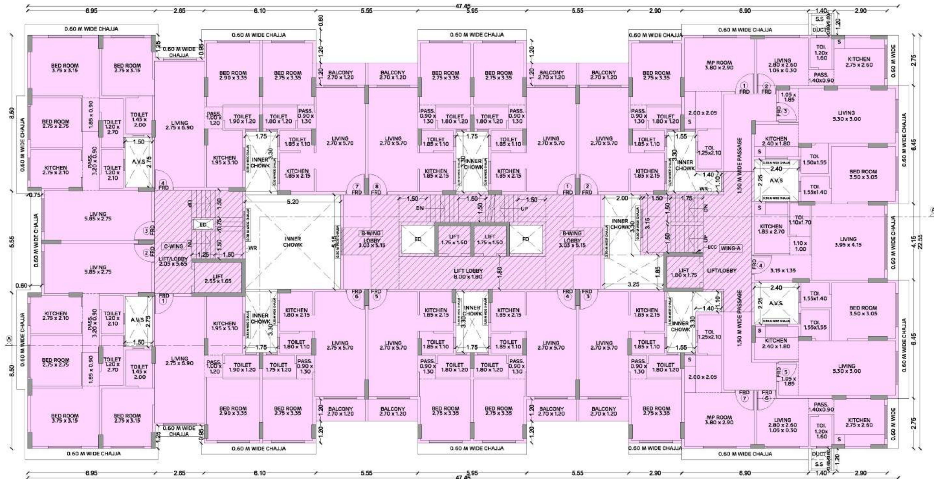
TYPICAL 2ND & 3RD FLOOR PLAN (SCALE - 1:100)
