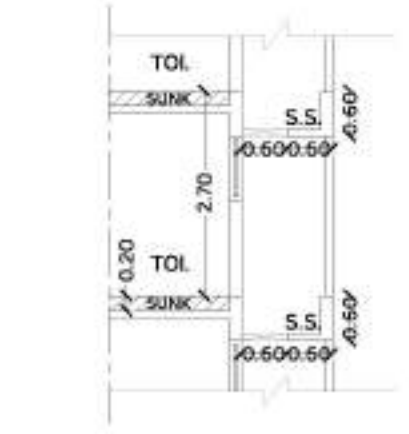
SECTION DETAIL FOR SERVICE DUCT (SCALE 1:100)
