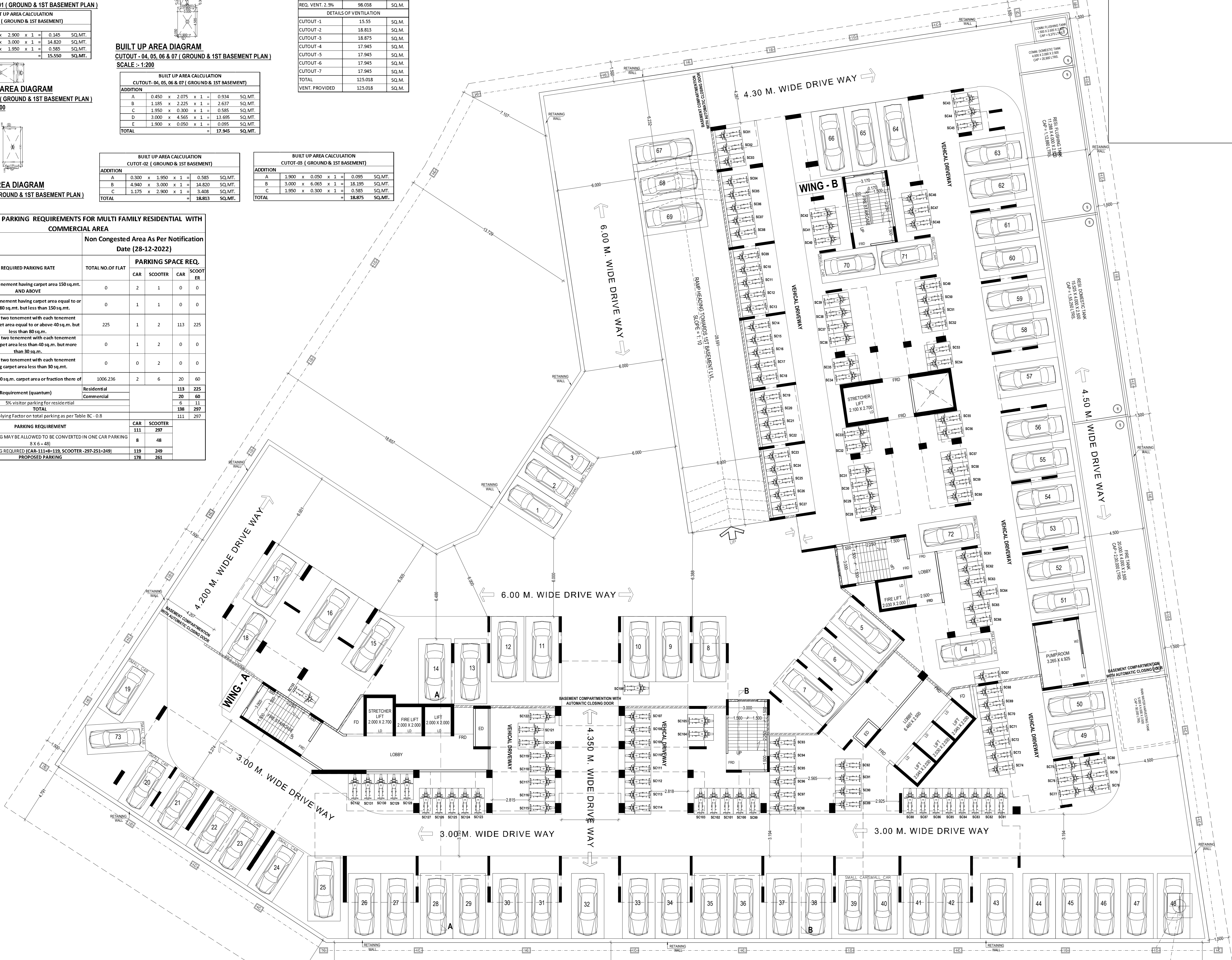
2ND BASEMENT PLAN SCALE :- 1:100 BIG CAR PARKING = 57 NOS. SMALL CAR PARKING = 16 NOS. SCOOTER PARKING = 133 NOS.
