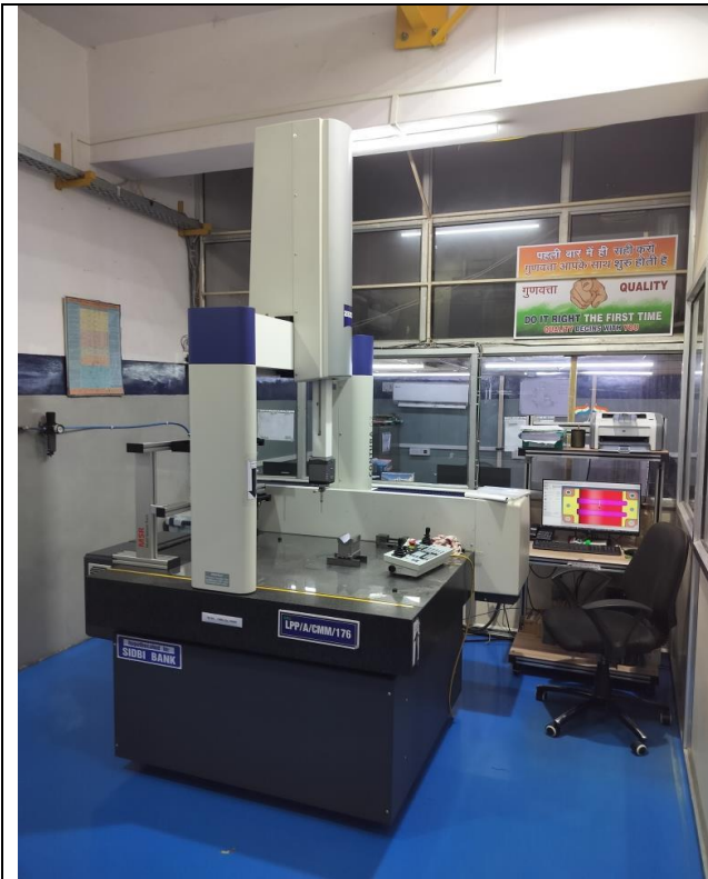
Carl Zeiss Make 3D CNC Co-Ordinate Measuring Machine, Model-Contura G2 7/10/6 Aktiv with Vast XTG D1 probe system along with standard accessories, Sr. No. 223705
