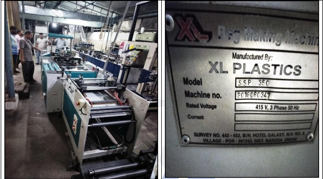
Three Side Seal Pouch making Machine, Model- SSP-350 Delta, Sr. No. 2018060347 at Location-2
