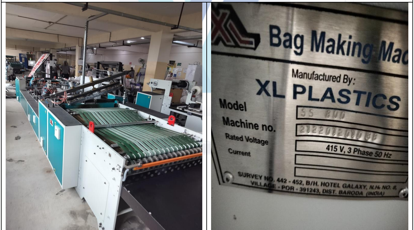
Side Seal Bag macking machine model SS 800 Delta, Sr. No. 212201201088 at Location-4
