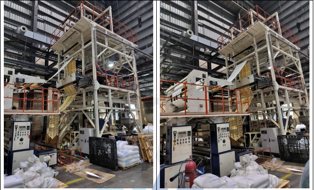
Three Layer Co Extrusion High Speed Inflation Machine KS CLFF45+50T at Location-4
