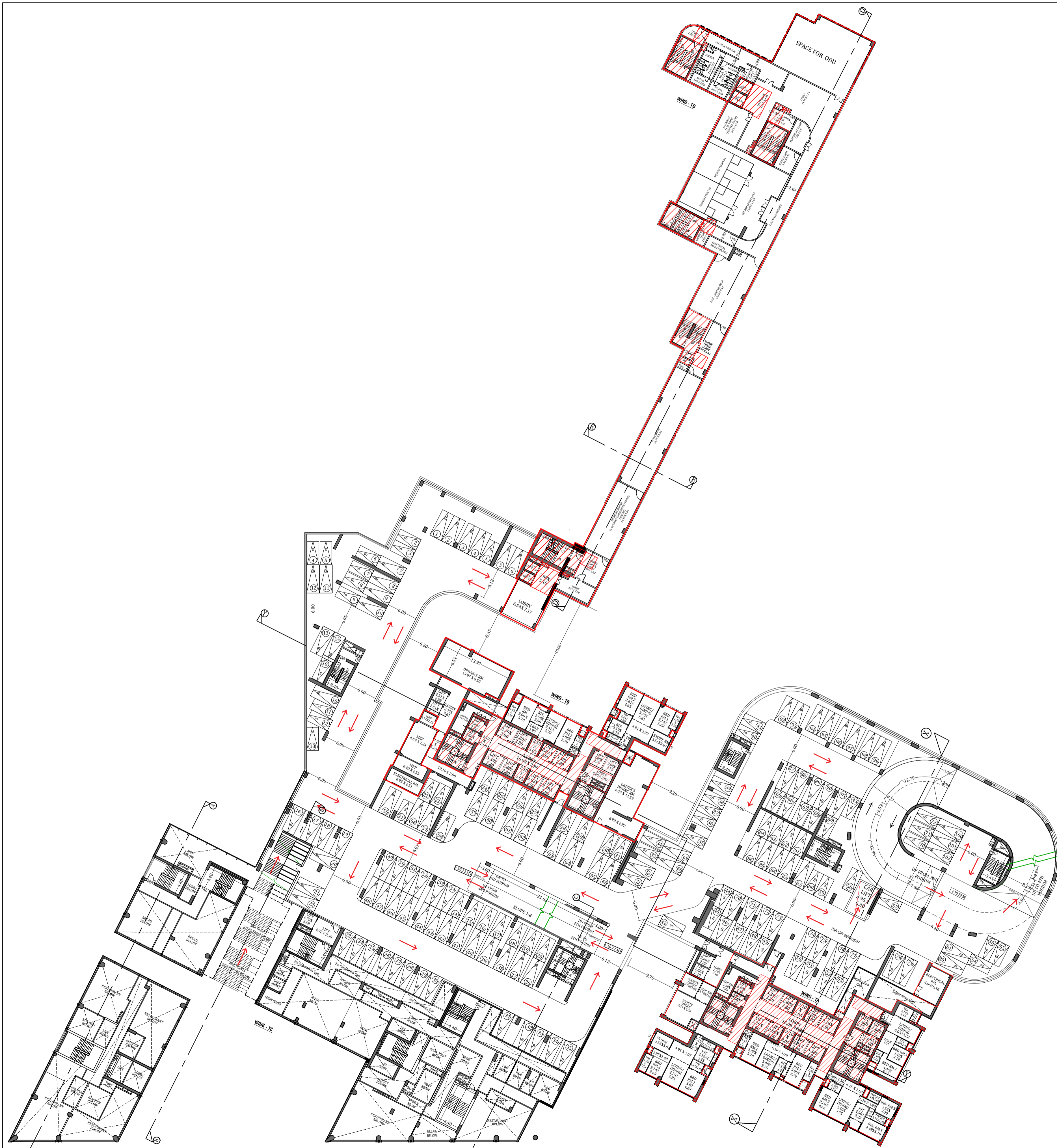
3RD MALL/PODIUM / RESIDENTIAL/ CLUBHOUSE-FITNESS CENTRE (FOR SOCIETY) FLOOR PLAN SCALE: 1:300 3RD MALL/PODIUM FLOOR (DCPR 2034) DIG PARKING = 102 SMALL PARKING = 72 TOTAL = 174
