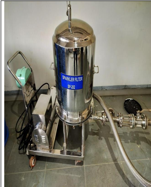
Zero Holdup Filter Press with SS 304 jacket, Size-14" X 10 "
