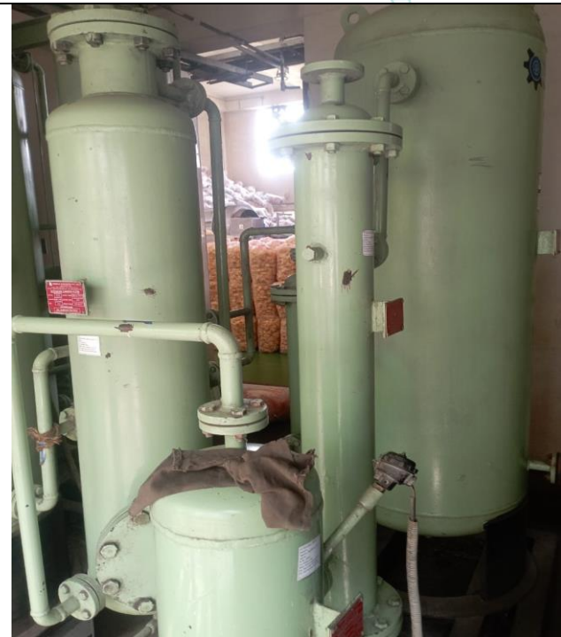
Nitrogen Plant, Capacity 25 m 3 /hr
