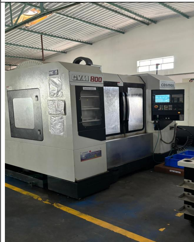
Used Cosmos make CNC Vertical Machining Centre, Model-CVM-800 with Siemens 828D CNC Controller ATC and other machine features, Sr. No. 08 0917 846, YOM-01/2018
