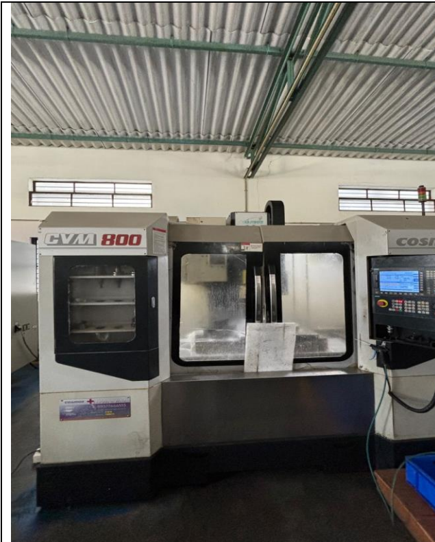
Used Cosmos make CNC Vertical Machining Centre, Model-CVM-800 with Siemens 828D CNC Controller ATC and other machine features, Sr. No. 08 1117 882, YOM-11/2017
