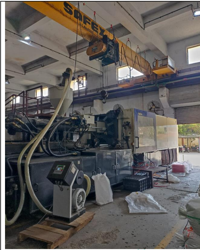
Windsor Make Fully Automatic Microprocessor Control Plastic Injection Moulding Machine, Model- Sprint-350, Sr. No. WC7930360
