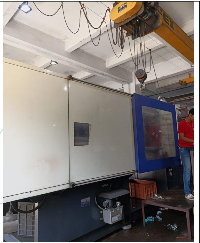
Windsor Make Fully Automatic Microprocessor Control Plastic Injection Moulding Machine, Model- Sprint-350, Sr. No. WC7930360
