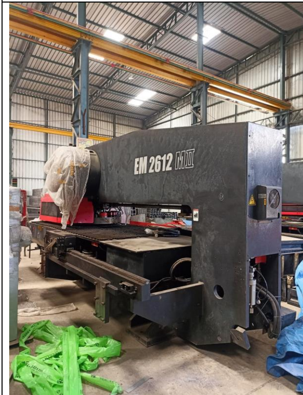
View of Amada CNC Turret Punch Press, Model- EM2612M2
