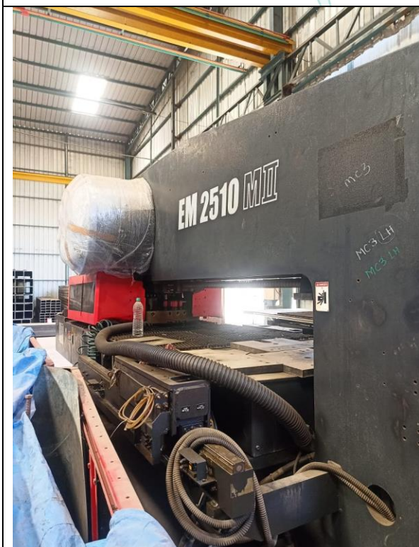
View of Amada CNC Turret Punch Press, Model- EM2510M2
