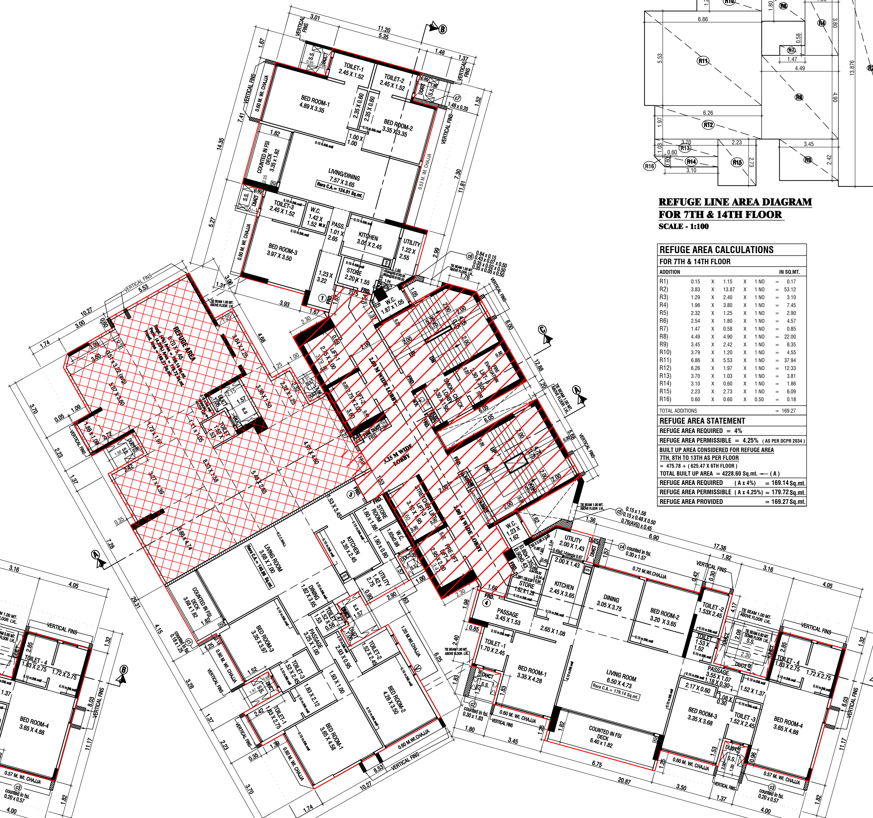
7TH & 14TH FLOOR PLAN (REFUGE) SCALE - 1:100
