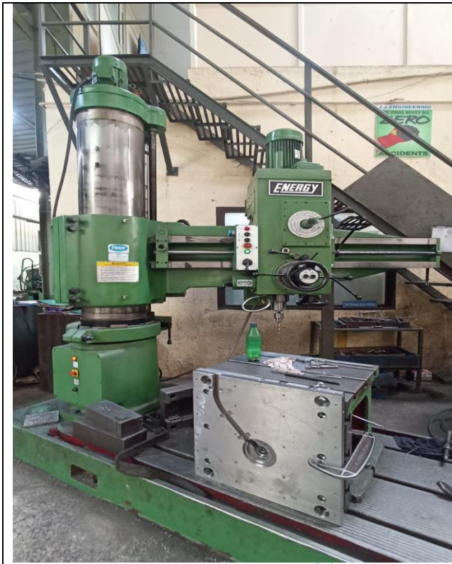
View of Energy Brand Radial Drilling Machine, Model : RDM - 50/1500 With Electro Mechanical Clamping Electricals And Standard Accessories
