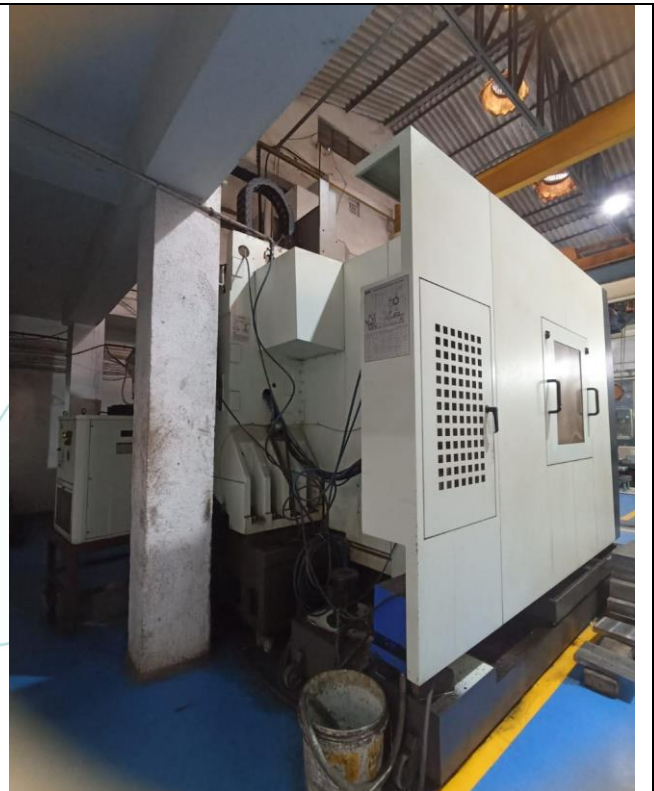
CNC Vertical Machining Centre, Model-BMV65 with Mitsubishi M80, Sr. No. 65156
