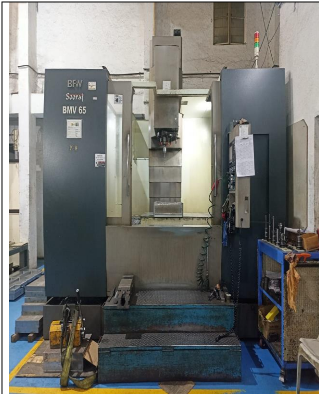
CNC Vertical Machining Centre, Model-BMV65 with Mitsubishi M80, Sr. No. 65156
