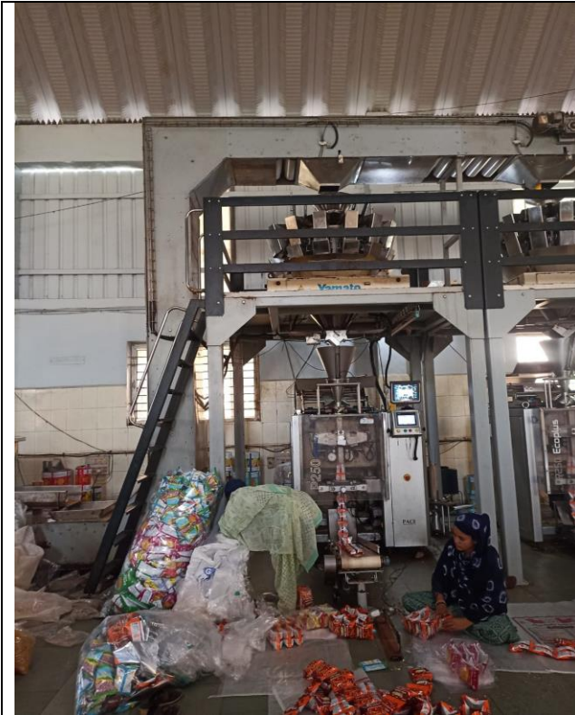
View of Pace Make High Speed Servo Driven Collar Type Vertical Form Fill Seal Machine with Accessories, Model No. P250 Eco+, Sr. No. SM-1769
