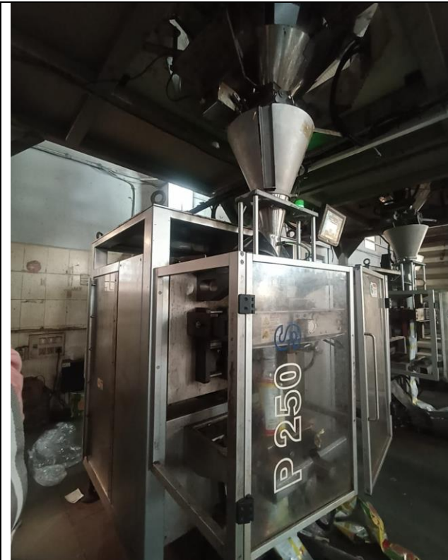
View of Pace Make High Speed Servo Driven Collar Type Vertical Form Fill Seal Machine with Accessories, Model No. P250 3S (ECO), Sr. No. SM-1176
