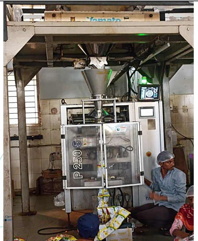
View of Pace Make High Speed Servo Driven Collar Type Vertical Form Fill Seal Machine with Accessories, Model No. P250 3S (ECO), Sr. No. SM-1176
