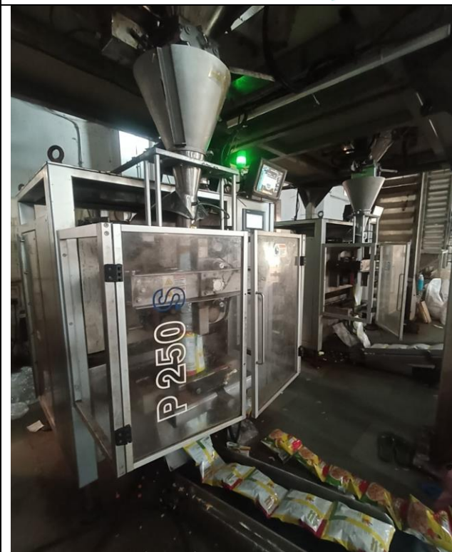
View of Pace Make High Speed Servo Driven Collar Type Vertical Form Fill Seal Machine with Accessories, Model No. P250 3S (ECO), Sr. No. SM-1176
