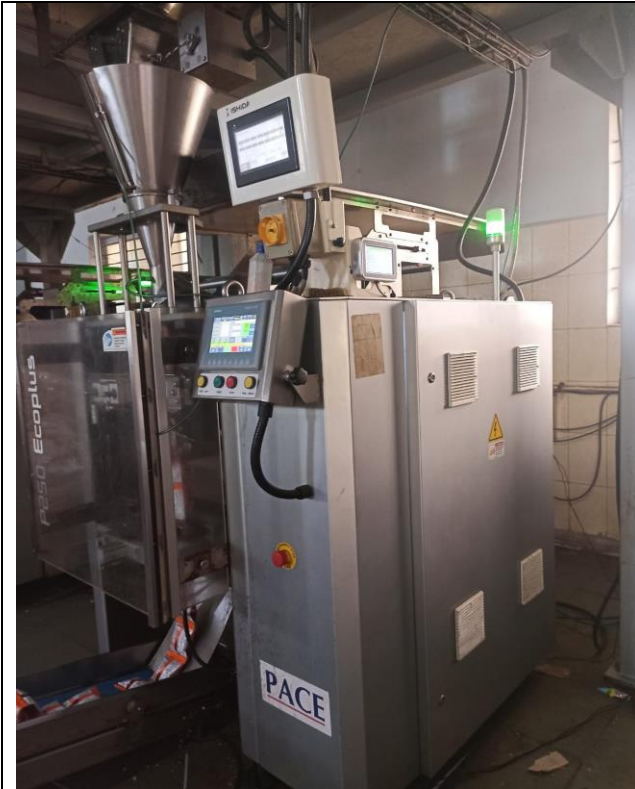
View of Pace Make High Speed Servo Driven Collar Type Vertical Form Fill Seal Machine with Accessories, Model No. P250 Eco Plus, Sr. No. SM-2414
