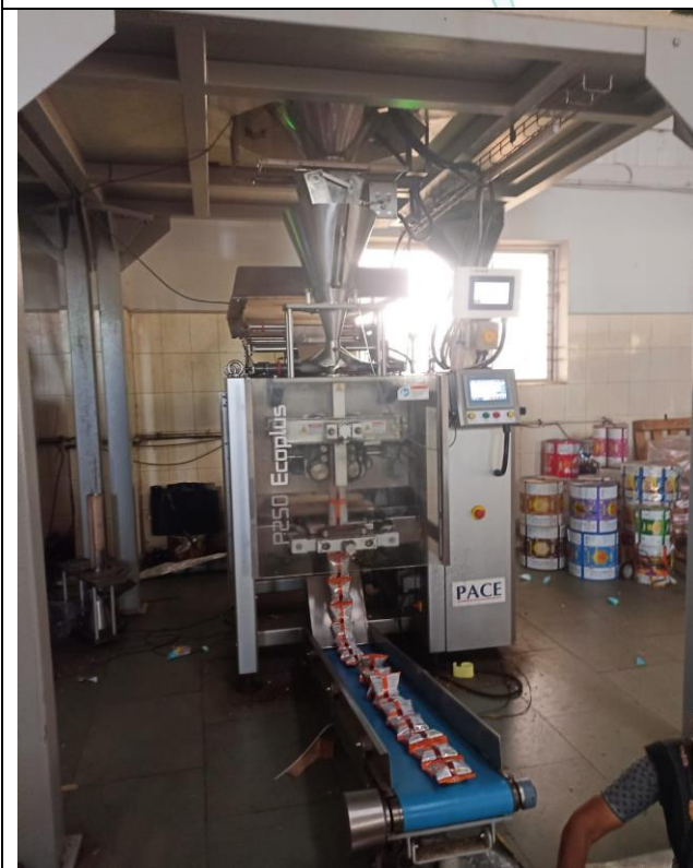
View of Pace Make High Speed Servo Driven Collar Type Vertical Form Fill Seal Machine with Accessories, Model No. P250 Eco Plus, Sr. No. SM-2414
