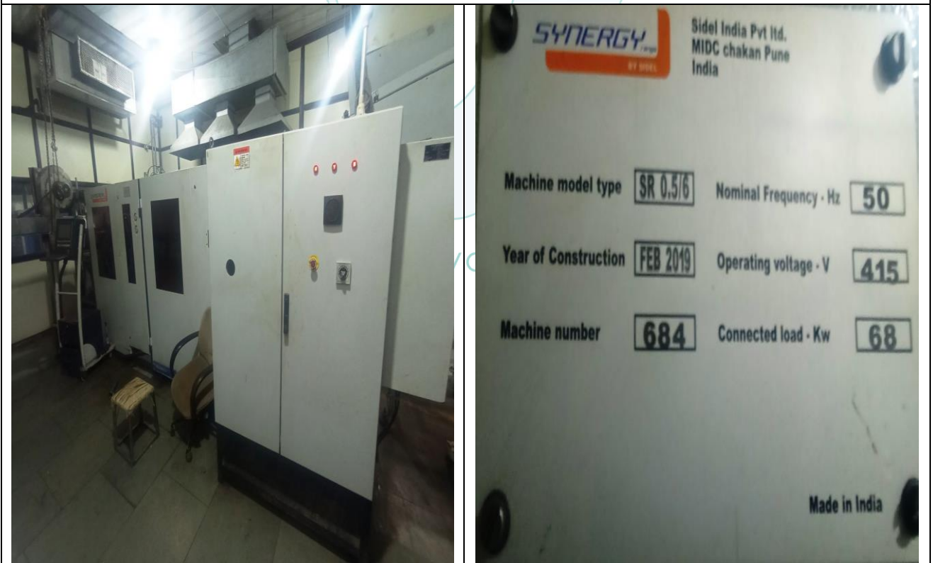
View of Synergy Model No. 0.5/6 Blowing Machine and Adaptation for 28 PCO 1881- Sr. No. 684
