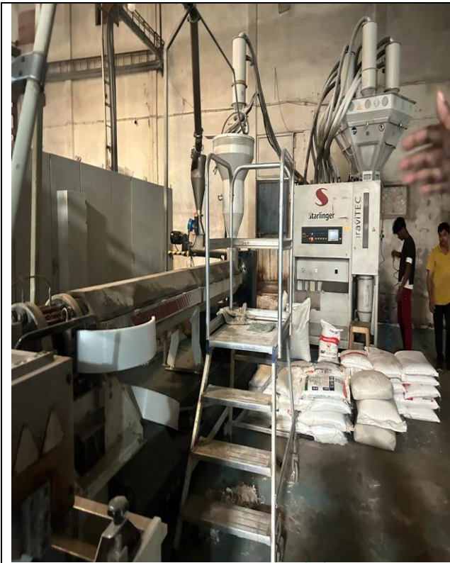
Tape Stretching Line starEX 1600ES 120/33 AC with Edge trim recycling with force feeding screw, stretching section with 8 godets, HP Oven, Automatic Knife bar changer, widening machine, and spare parts, Sr. No. 17-00274-1
