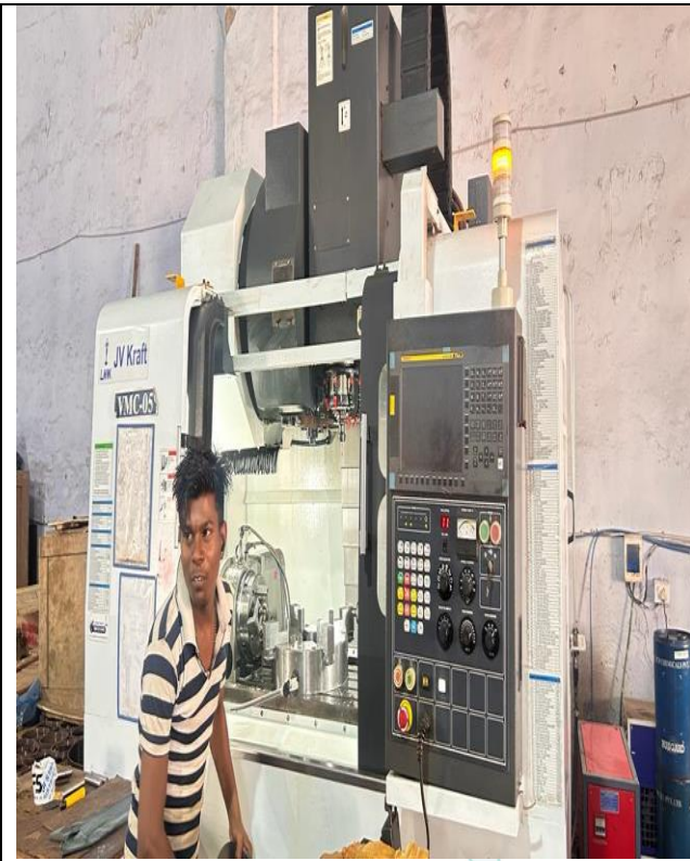
JV Kraft CNC Vertical Machining Centre-Fanuc, Serial No. V320-00662 installed at Unit-II
