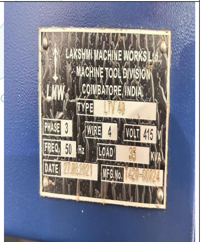
LTV 40 CNC Vertical Turret Lathe-Fanuc, Serial No. L420-00024 installed at Unit-II
