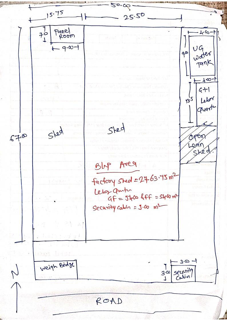
Factory - Shed pcc feoting, ms framed structure, que sheet soof, Trionix flooring,
