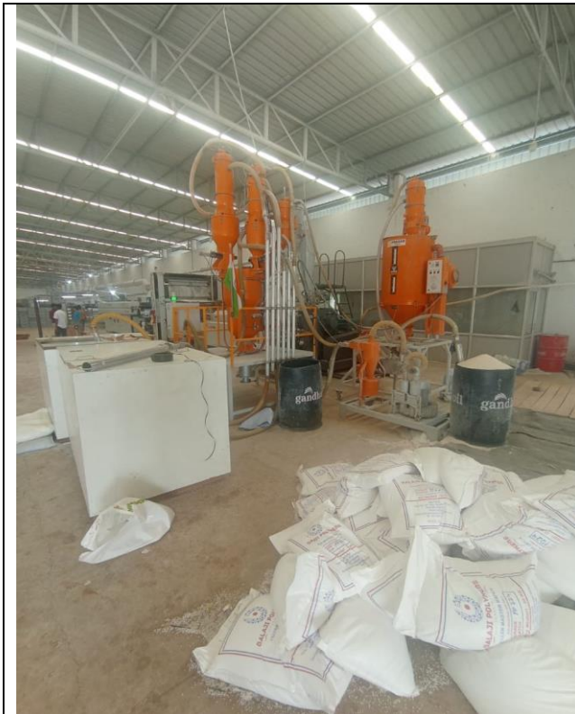
Gravimetric Dosing Mixing Conveying System Five Components Offline GV-200 Sr. No. 631 & Hot Air Dryer for filler drying with accessories
