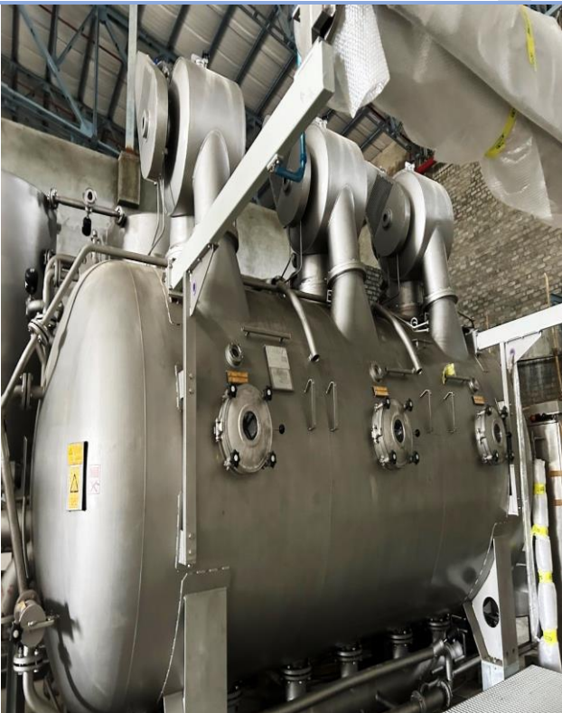
View of FABRIC DYEING MACHINE 1200KG, Model- TOWELTEC3-3T, Sr. No. 47040853
